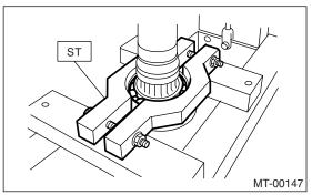
2) Do not disassemble the center differential except ball bearing part because it is a non-disassemble part.
