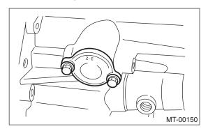
2) Install the reverse check ball, reverse accent spring, gasket and plug to transfer case.
