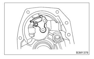
2) Install reverse check sleeve assembly to transfer case.
