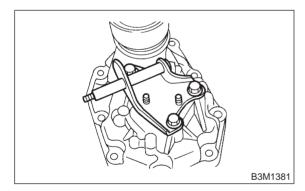
4) Install transfer drive gear to extension case.
