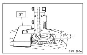
9) Calculate space "U" using the following equation: U = S + T - 0.24 mm (0.0094 in) [Thickness of gasket]
