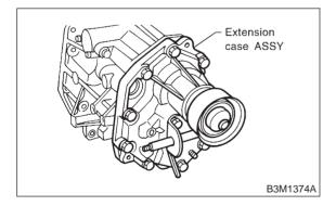
2) Remove transfer driven gear and center differential as a set.
