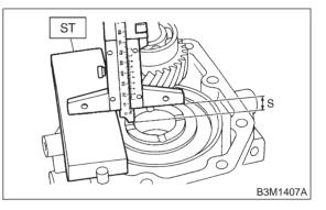
8) Measure depth "T" between extension case and transfer drive gear.
