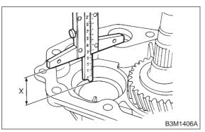
4) Calculate space "Y" using the following equation: Y = X - W + 0.24 mm (0.0094 in) [Thickness of gasket]
