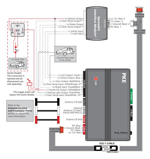
······ These wires are **not** required in D2D mode.
