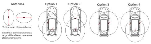
**Note**: An optionnal 12-foot antenna (part# SANT-PKE12) can be installed to increase the active zone coverage. When a third antenna is installed, feature 4, option 2 must be enable through the "Features and Options List" section on page 21.
