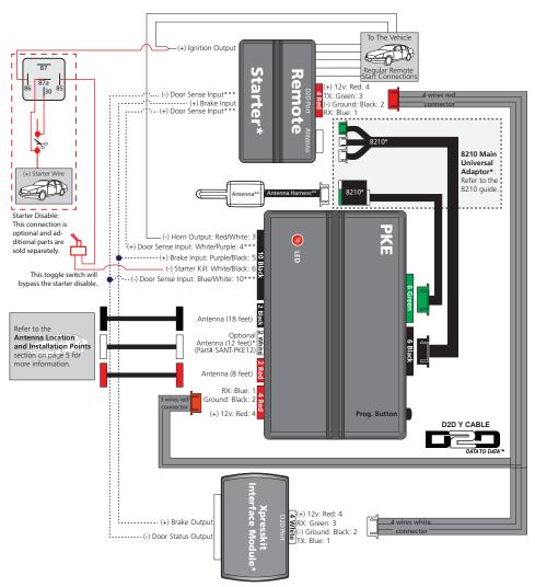
······ These wires are **not** required in D2D mode.
