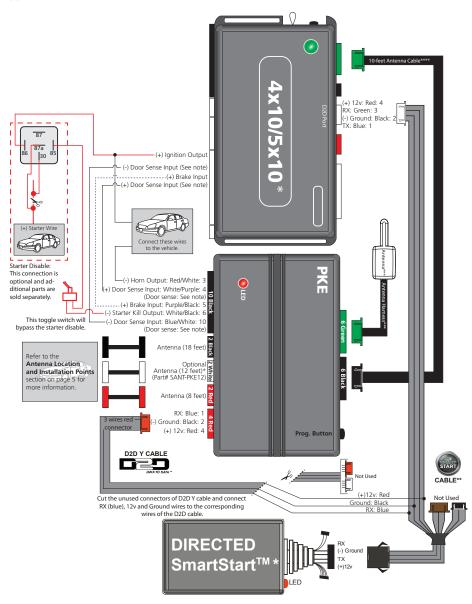
······ These wires are not required in D2D mode.
