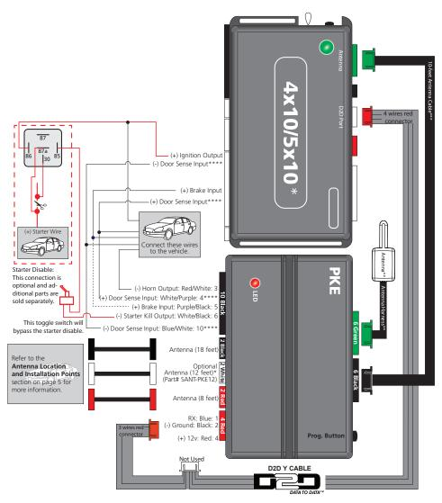
······ These wires are **not** required in D2D mode.
