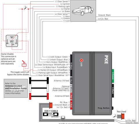
Cut the 4-wire red connector of D2D Y-cable and connect 12v and Ground wires to the corresponding wires of the DIRECTED SmartStart™ cable.
