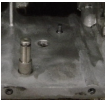
Looking inside the case (left), you can see the small anchor above and to the right of the shift lever anchor and the reverse light switch hole...
