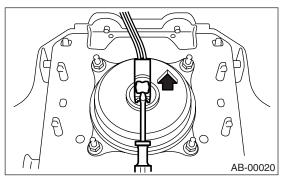
(2) Pull the connector to disconnect from driver's side airbag module assembly.
