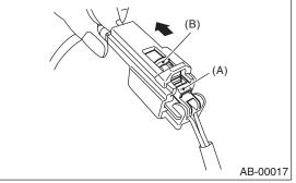
(3) With the slide lock pulled, remove the lock arm to its original position, and then pull in the direction of the arrow and separate the connector.
