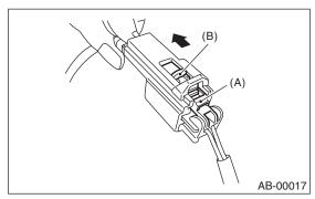
(3) With the slide lock pulled, remove the lock arm to its original position, and then pull in the direction of the arrow and separate the connector.
