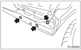
4) When removing the rear bumper beam assembly, remove the six bolts on bumper stay.
