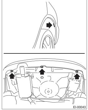
3) Remove the clips from bumper and bracket.
