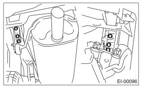
5) Remove the rear combination light assemblies from each side. <Ref. to LI-18, REMOVAL, Rear Combination Light Assembly.>
