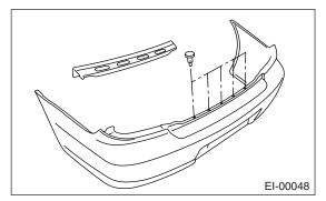
12) Remove the four bolts to remove side bracket and bumper stay.
