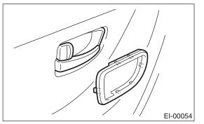
3) Remove the power window control switch. <Ref. to GW-7, REMOVAL, Power Window Control Switch.>
