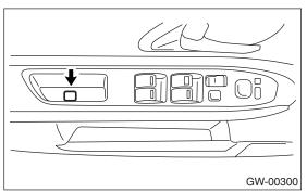
3) Loosen the screw to remove the power window main switch.
