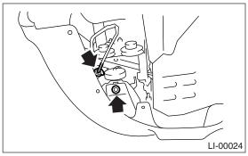
5) Remove the mounting bolts and clip, and then detach the fog light assembly.
