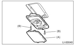
3) Disconnect the harness connectors and remove the light.
