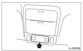
3) Remove the spot map light installation screws.
