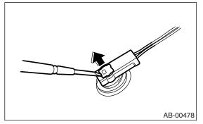
(2) Pull the connector to disconnect from retractor assembly.
