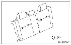
4) Remove the hog rings (A) from around the seat cushion.
