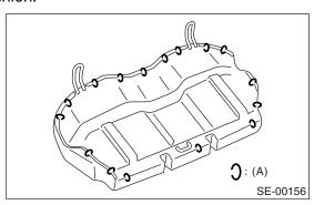
5) Remove the hog rings (A), and then remove the cover.
