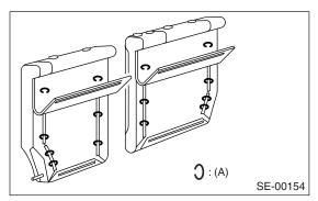
3) Remove the hog rings (A) on front side of cushion pad, and then remove the cover.
