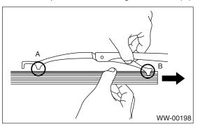
2) Insert the wiper rubber top until it protrudes about 20 mm (0.79 in) from the stopper (D).
