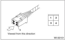
• The number of poles or pins, presence of a lock, and pin number of each terminal are indicated in the sketch of each connector. In the sketch, the highest pole number refers to the number of poles which connector has. For example, the sketch of connector shown in the figure indicates the connector has 9 poles.
