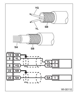
• The wire color code, which consists of two letters (or three letters including Br or Lg), indicates the standard color (base color of the wire covering) by its first letter and stripe marking by its second letter.
