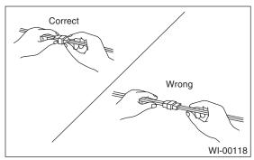
5) Some connectors are provided with a lock. One type of such a connector is disconnected by pushing the lock, and the other, by moving the lock up. In either type the lock shape must be identified before attempting to disconnect the connector.
