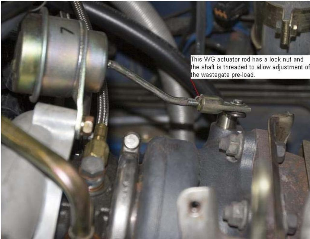
The location of the threads can be located at either end of the wastegate actuator rod, see the below picture where it demonstrates the threaded section is closest to the WG actuator diaphragm.
