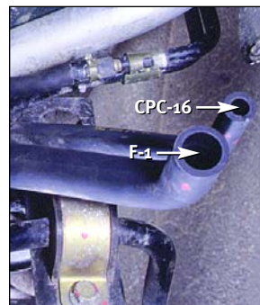
Purge (CPC-16) and Fuel (F-1) Hoses
