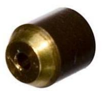
The restrictor pill should fit tightly inside the vacuum line and should have the hole machined in the center of the pill.
