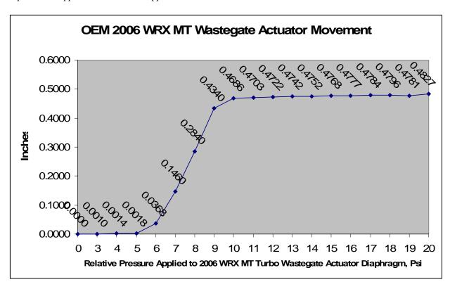
NOTE: The MORE boost you run, the LESS wastegate you need/use. So unless you want to run less pressure than stock and/or have un-tunable boost problems, we suggest that you do not port your wastegate by hand. We suggest you leave your wastegate, the area around it, the turbine housing, etc. alone and tune your boost curve through the proper means.
