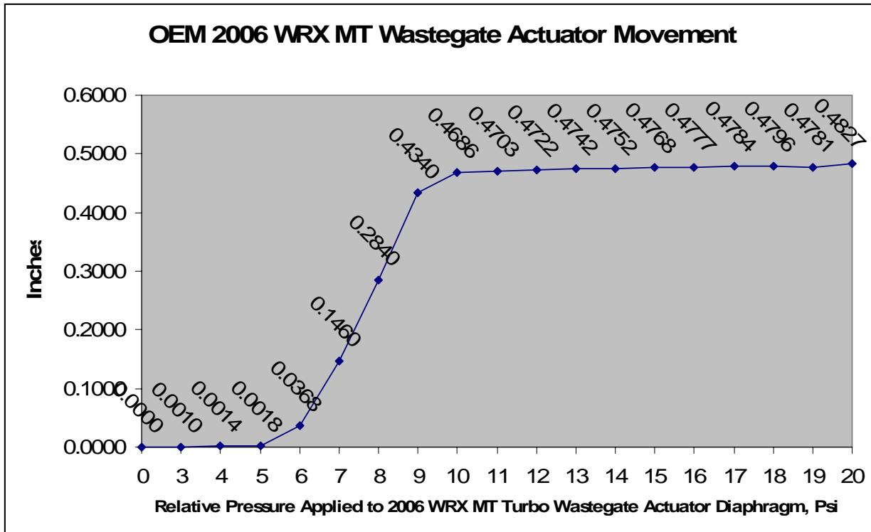
NOTE: The MORE boost you run, the LESS wastegate you need/use. So unless you want to run less pressure than stock and/or have un-tunable boost problems, we suggest that you do not port your wastegate by hand. We suggest you leave your wastegate, the area around it, the turbine housing, etc. alone and tune your boost curve through the proper means.
