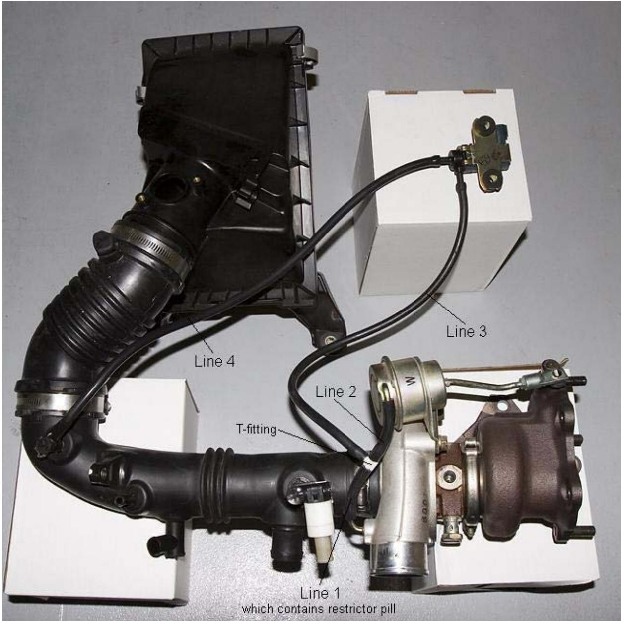
Line 1 plumbs the compressor housing to one end of the T-fitting. This line contains the brass restrictor pill.
