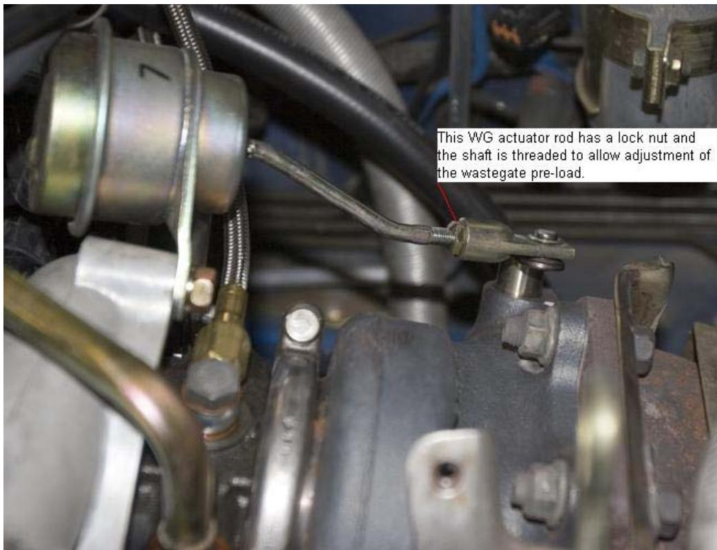
This WG actuator rod has a lock nut and the shaft is threaded to allow adjustment of the wastegate pre-load.
