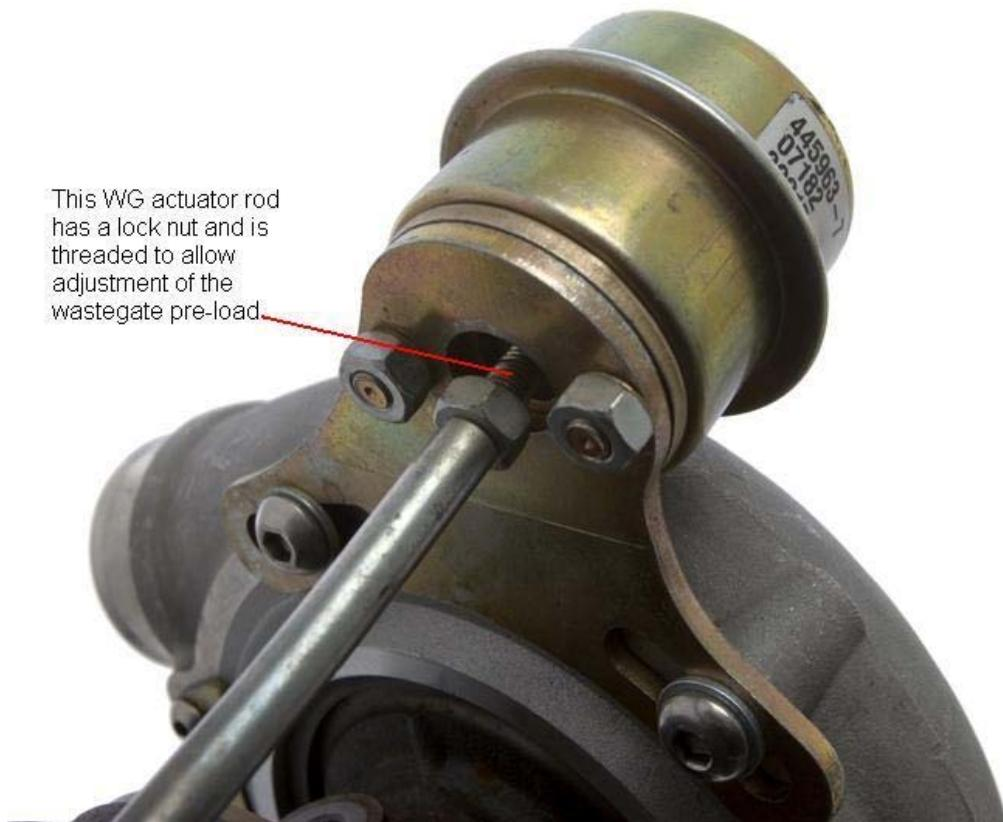
This WG actuator rod has a lock nut and is threaded to allow adjustment of the wastegate pre-load.
