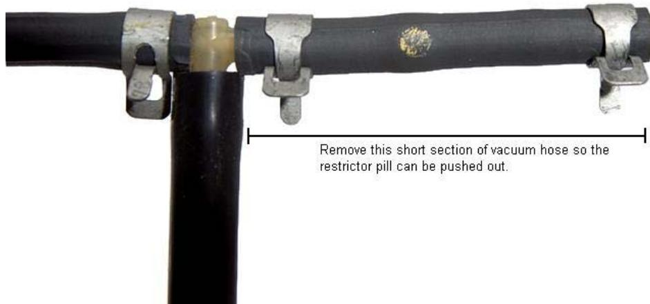
Carefully insert straight pick into the center of the restrictor pill and gently push out the brass restrictor pill. Be sure not to poke or rip the vacuum hose.
