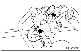
9) Remove the pressure control solenoid valve from bracket.
