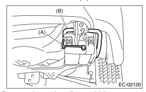
7) Remove the canister from vehicle.
