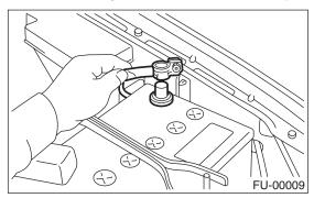
2) Disconnect the connector and hoses of purge control solenoid valve, and then remove the purge control solenoid valve.
