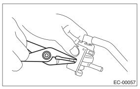
10) Disconnect the vacuum hose from pressure control solenoid valve.
