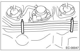
5) Remove the bolt and nut which hold the fuel tank pressure sensor onto the bracket.
