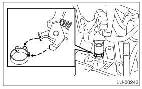
2) Install the intake manifold.
