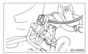
7) Disconnect the two evaporation hoses from pressure control solenoid valve.
