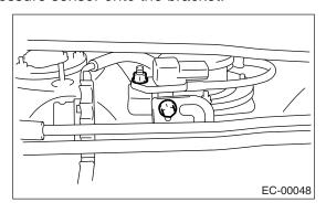
6) Disconnect the pressure hose from fuel tank pressure sensor.
