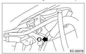
6) Disconnect the connector from pressure control solenoid valve.
