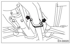
2) Remove the rubber cushions, and detach the muffler.
