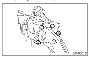
4) Install the center exhaust pipe to rear exhaust pipe.
