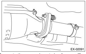
4) Separate the rear exhaust pipe from muffler.
