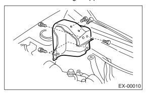
10) Remove the bolts which install the upper side of turbocharger lower cover, and remove it.
