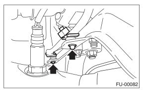
7) Tighten the bolt which holds the center exhaust pipe bracket to transmission.
