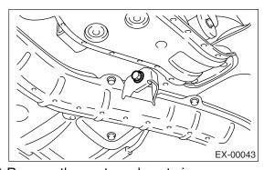
19) Remove the center exhaust pipe.
