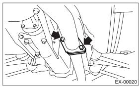
5) Remove the rear exhaust pipe.
