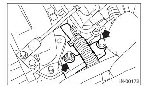
7) Connect the engine coolant hose which is connected to coolant filler tank.
