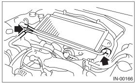
2) Remove the air by-pass valve from intercooler.
