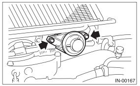
2) Disconnect the air by-pass hoses from air by-pass valve.
