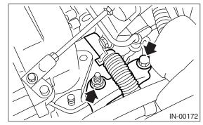
12) Disconnect the oil outlet hose from pipe.
