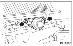
3) Remove the bolts which secure the intercooler to bracket.
