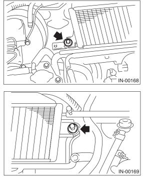
4) Remove the intercooler air duct from turbocharger.
