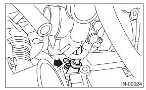
13) Take out the turbocharger from engine compartment.
