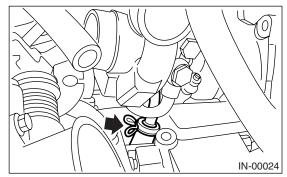
2) Install the turbocharger to intake duct.
