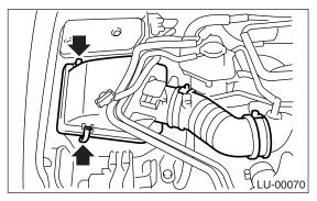
16) Connect the connector to mass air flow sensor.
