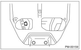
3) Replace the drain plug gasket.
