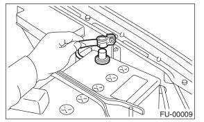
4) Disconnect the connector from mass air flow sensor.
