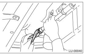
6) Remove the engine oil filter. <Ref. to LU(H4DOTC)-20, REMOVAL, Engine Oil Filter.>7) Remove the connector, and then remove the oil cooler.
