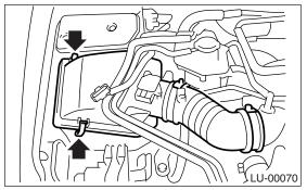
6) Remove the intercooler. <Ref. to IN(H4DOTC)-10, REMOVAL, Intercooler.> 7) Remove the pitching stopper.
