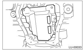
Install the oil strainer onto baffle plate.
