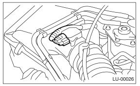
5) Remove the air intake boot and air cleaner upper cover.
