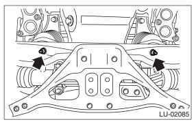
8) Install the front exhaust pipe assembly. <Ref. to EX(H4DOTC)-6, INSTALLATION, Front Exhaust Pipe.>
