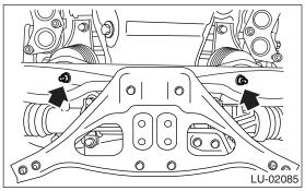
15) Remove the bolts which install the oil pan on cylinder block while raising up engine.
