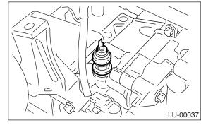
3) Connect the terminal of oil pressure switch.
