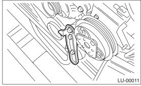
10) Remove the crank pulley by using ST. <Ref. to ME(H4DOTC)-45, REMOVAL, Crank Pulley.>
