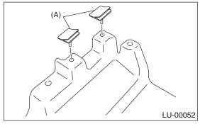
2) Install the baffle plate.
