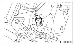
3) Remove the oil pressure switch.
