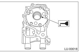
4) Be careful not to scratch the oil seal when installing the oil pump on cylinder block.
