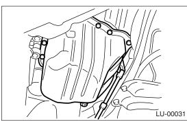
6) Lower the engine onto front crossmember.7) Tighten the nuts which install the front cushion rubber onto front crossmember.
