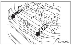
14) Install the intercooler. <Ref. to IN(H4DOTC)-10, INSTALLATION, Intercooler.>
