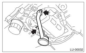
18) Remove the baffle plate.
