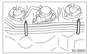
5) Remove the nuts and bolts which install the fuel tank pressure sensor on bracket.
