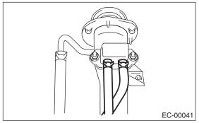
3) Remove the shut valve from fuel filler pipe.
