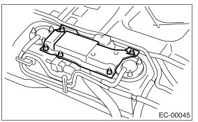
3) Disconnect the connector from fuel tank pressure sensor.
