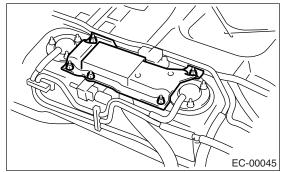
3) Disconnect the connector from fuel tank sensor control valve.
