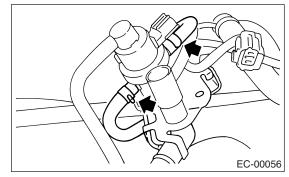
9) Remove the pressure control solenoid valve from bracket.
