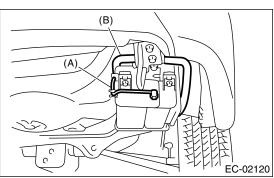
7) Remove the canister from vehicle.
