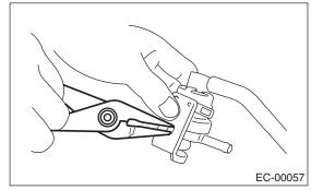
10) Disconnect the vacuum hose from pressure control solenoid valve.
