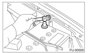
2) Disconnect the connector and hoses of purge control solenoid valve, and then remove the purge control solenoid valve.
