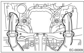
8) Remove the bolt which installs the front and center exhaust pipe assembly to hanger bracket.
