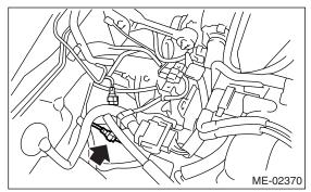
3) Disconnect the rear oxygen sensor connector.
