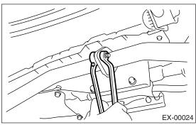
4) Install the rear exhaust pipe to center exhaust pipe.
