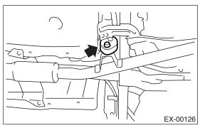
3) Install the rear exhaust pipe to muffler.
