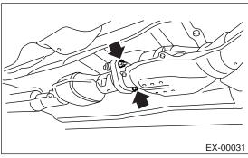
8) Tighten the bolt which holds the front and center exhaust pipe assembly to hanger bracket.
