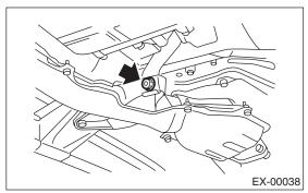
9) Remove the front and center exhaust pipe assembly from vehicle.
