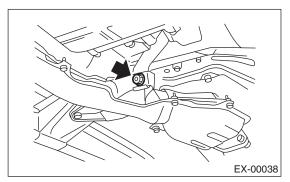
5) Tighten the nuts which hold the front exhaust pipe onto cylinder heads.
