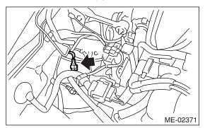
11) Connect the front oxygen (A/F) sensor connector.
