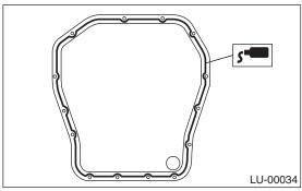
5) Tighten the bolts which install the oil pan onto engine block.
