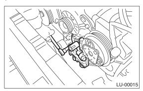
14) Remove the oil pump by using flat tip screwdriver.
