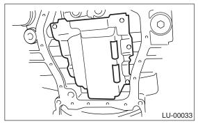
3) Install the oil strainer onto baffle plate.
