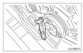
9) Remove the crankshaft pulley by using ST.
