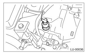
3) Remove the oil pressure switch.
