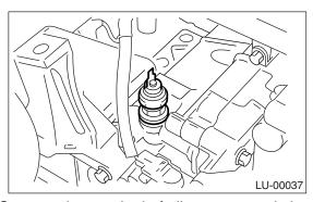
3) Connect the terminal of oil pressure switch.
