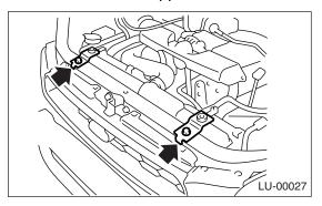
8) Support the engine with a lifting device and wire ropes.
