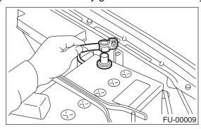
18) Fill engine oil. <Ref. to LU(H4SO)-9, INSPECTION, Engine Oil.>
