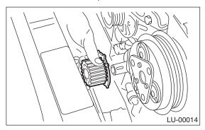
13) Remove the bolts which install the oil pump onto cylinder block.
