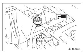
2) Install the oil pressure switch onto engine block.
