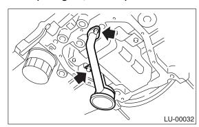
4) Apply liquid gasket to the mating surfaces, and then install the oil pan.
