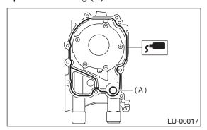
3) Apply a coat of engine oil to the inside of oil seal.
