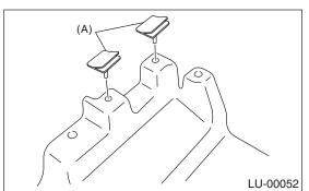
2) Install the baffle plate.
