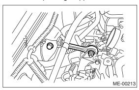
20) Disconnect the fuel delivery hose (A), return hose (B) and evaporation hose (C). <Ref. to FU(H4SO)-56, REMOVAL, Fuel Delivery, Return and Evaporation Lines.>
