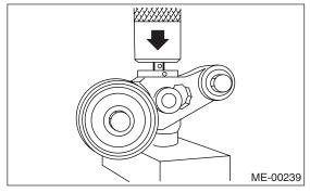
(3) With a 2 mm (0.08 in) dia. stopper pin or a 2 mm (0.08 in) (nominal) dia. hex wrench inserted into the stopper pin hole in cylinder, secure the adjuster rod.
