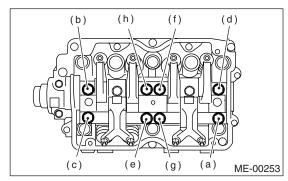
(2) Remove the valve rocker assembly.
