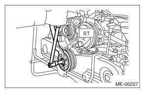
3) Remove the crank pulley.
