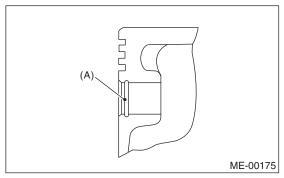
5) Check the piston pin snap ring for distortion, cracks and wear.
