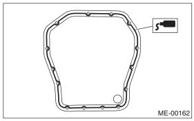
25) Apply liquid gasket to the mating surfaces and threaded portion of bolt (A) as shown in the figure, and then install the oil separator cover.
