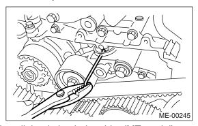
6) Install the timing belt guide. (MT model)
