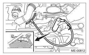
If the timing is not correct, check the ignition control system. <Ref. to EN(H4SO)(diag)-2, Basic Diagnostic Procedure.>
