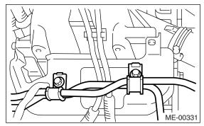
(4) Connect the power steering switch connector.
