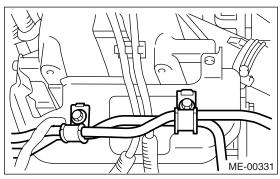
(3) Remove the bolts which install the power steering pump to bracket.
