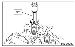
(5) Compress the valve spring and fit the valve spring retainer key.
