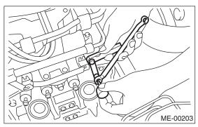
3) Adjust the valve clearance in #3, #2 and #4 cylinder in the same adjustment procedure as #1 cylinder.
