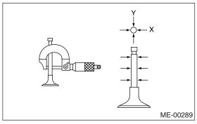
2) If the clearance between valve guide and stem exceeds the standard value, replace the valve guide or valve itself whichever shows greater amount of wear. See the following procedure for valve guide replacement.
