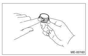
(6) Install the service hole plug and gasket.
