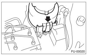
(5) Place the power steering pump on right side wheel apron.
