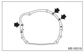
24) Set the ST to converter case. (AT model) ST 498277200 STOPPER SET
