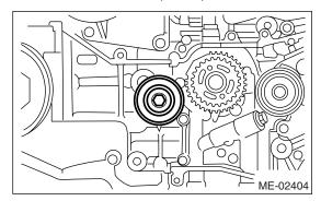
2) Remove the automatic belt tension adjuster assembly.
