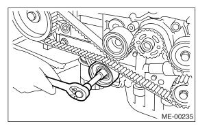
5) After ensuring the marks on timing belt and cam sprockets are aligned, remove the stopper pin from belt tension adjuster.
