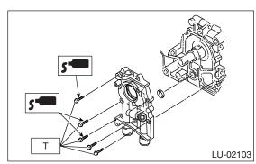
30) Install the water pump and gasket.
