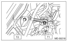
8) Remove the ST from converter case. (AT model)
