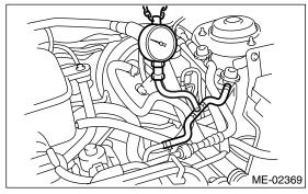
4) Connect the connector of fuel pump relay.
