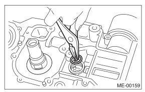
(5) Apply liquid gasket around the service hole plug.
