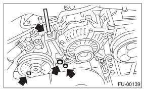
(4) Remove the power steering tank from bracket by pulling it upward.
