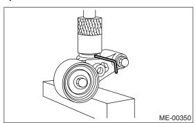
2) Install the automatic belt tension adjuster assembly.
