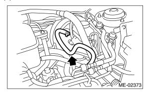
(2) Heater inlet and outlet hoses
