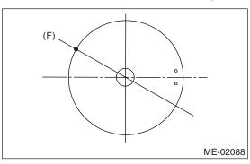
16) Position the lower rail gap at 120° on counter-clockwise of (C) that shown (G) in the figure.
