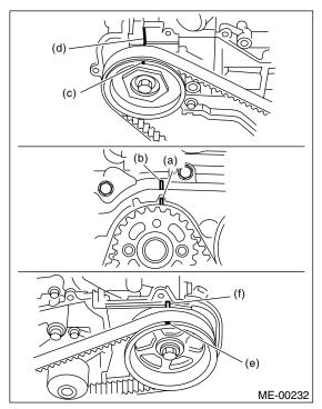
(2) Using white paint, put alignment marks or arrow marks on the timing belts in relation to the crank sprocket and cam sprockets.
