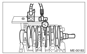
3) Inspect the crank journal and crank pin for wear. If they are not within the specifications, replace the bearing with a suitable (undersize) one, and replace or recondition crankshaft as necessary. When grinding the crank journal or crank pin, finish them to the specified dimensions according to the undersize bearing to be used.
