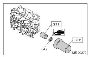
4) Install the plug using ST.
