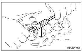
(8) Recheck the contact condition between valve and valve seat after replacing the valve guide.
