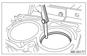
4) Measure the clearance between piston ring and piston ring groove with a thickness gauge.
