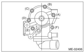
20) Remove the oil pump from cylinder block. Use a flat tip screwdriver as shown in the figure when removing the oil pump.
