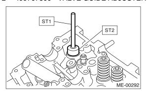
(6) Check the valve guide protrusion.
