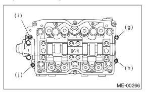
(3) Install the valve rocker assembly.
