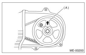
10) Measure #1 cylinder valve clearance using thickness gauge.
