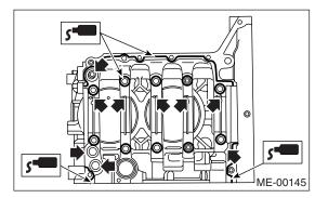
3) Tighten the 10 mm cylinder block connecting bolts on LH side (A — D) in alphabetical sequence.
