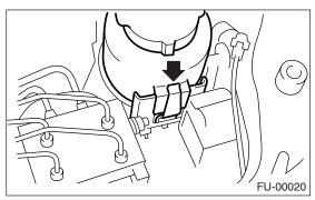
(2) Install the power steering pump on bracket, and tighten the bolts.
