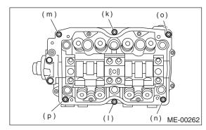
(4) Remove the camshaft cap.
