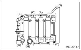
10) Install the rear oil seal using ST1 and ST2.ST1 499597100 OIL SEAL GUIDEST2 499587200 OIL SEAL INSTALLER
