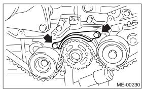
(2) Check and adjust the clearance between timing belt and timing belt guide by using thickness gauge.
