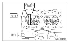
(3) Turn the cylinder head upside down and place the ST as shown in the figure.
