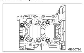
9) Tighten the 8 mm and 6 mm cylinder block connecting bolts on LH side (A — H) in alphabetical sequence.
