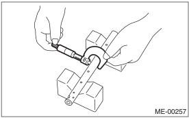
2) If the oil clearance exceeds the limit, replace the valve rocker arm or shaft, whichever shows greater amount of wear.
