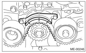
(3) Tighten the timing belt guide mounting bolts.
