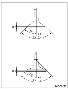
2) Put a small amount of grinding compound on the seat surface and lap the valve and seat surface. <Ref. to ME(H4SO)-56, VALVE SEAT, INSPECTION, Cylinder Head.> Install a new intake valve oil seal after lapping.
