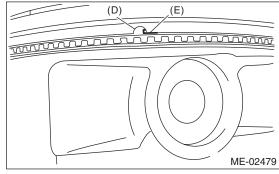
15) Position the expander gap at 180° on the reverse side of (C) that shown (F) in the figure.
