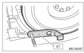
27) Install the drive plate.To lock the crankshaft, use the ST.
