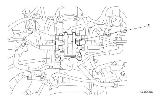
(1) Ignition coil and igniter assembly
