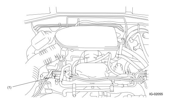
(1) Ignition coil and igniter assembly
