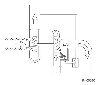
When the supercharging pressure reaches the predetermined level, the wastegate controller lets the supercharging pressure press the diaphragm. This causes the wastegate valve to open through a linkage. With the wastegate valve open, part of the exhaust gas is allowed to flow into the exhaust gas pipe that bypasses the passage to the turbine.
