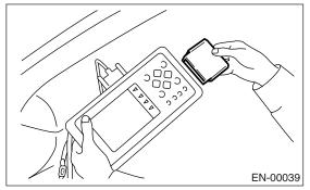
6) Connect the test mode connector (A) at the lower portion of instrument panel (on the driver's side).
