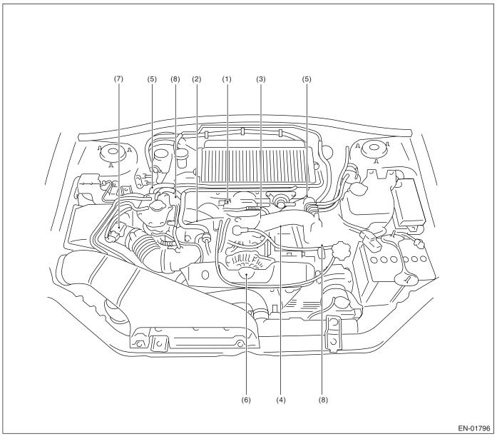
Manifold absolute pressure sensor (1) (2) Engine coolant temperature sen-
