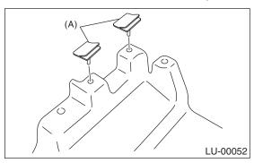
2) Install the baffle plate.
