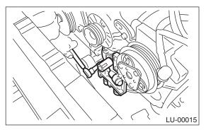
15) Remove the oil pump using flat tip screwdriver.
