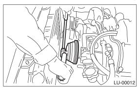
11) Remove the water pump. <Ref. CO(H4DOTC)-19, REMOVAL, Water Pump.>
