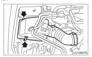
16) Connect the connector to mass air flow and intake air temperature sensor.
