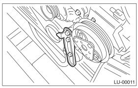
10) Remove the crank pulley by using ST. <Ref. to ME(STi)-42, REMOVAL, Crank Pulley.>
