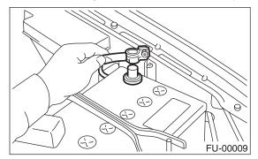
4) Disconnect the connector from mass air flow and intake air temperature sensor.
