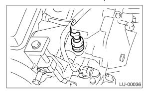
3) Remove the oil pressure switch.
