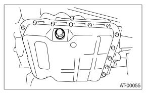
6) Replace the gasket with a new one, and then tighten the drain plug.
