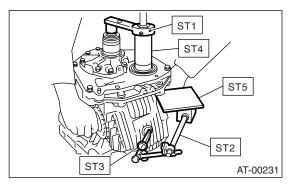
9) Adjust the tooth contact between front differential and drive shaft. <Ref. to 4AT-110, ADJUST-MENT, Drive Pinion Shaft Assembly.>
