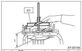
2) Using the ST, measure the distance from the oil pump housing mating surface to the end surface of ST.
