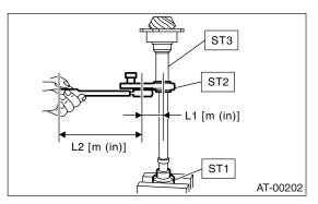
6) Measure the starting torque of the bearing. Make sure the starting torque is within the specified range. If out of the allowable range, replace the roller bearing.
