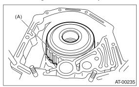
(A) High clutch and reverse clutch ASSY
