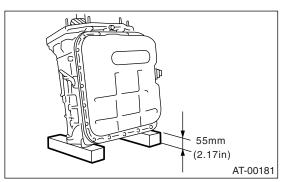
15) Remove the oil pump housing and adjusting thrust washer.
