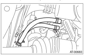
7) Remove ATF cooler pipe from frame.
