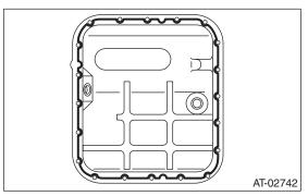
7) Apply liquid gasket fully to three holes other than screw holes on transmission case.
