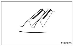
Corrective action: Increase thickness of drive pinion height adjusting washer in order to bring drive pinion close to hypoid driven gear.
