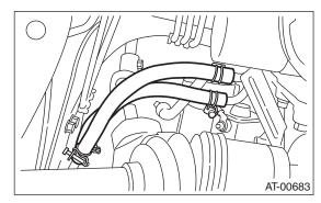
4) Connect ATF cooler hose to pipe of radiator side.
