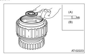
15) Install the rear sun gear in proper direction.
