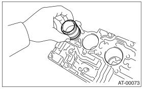
4) Install the spring and four steel balls to specified positions of upper valve body.
