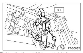
4) Tighten the three inhibitor switch bolts.
