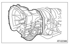
9) Remove the seal pipe if it is attached. (Reusing is not allowed.)
