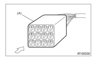
(A) Inhibitor switch connector
