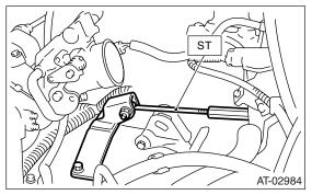
16) Remove the bolt which holds the upper side of transmission to engine.
