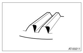
Corrective action: Increase thickness of drive pinion height adjusting washer in order to move drive pinion close to hypoid driven gear.
