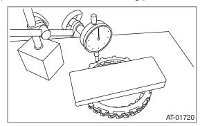
12) Using the following formula, calculate N indicated on the push/pull gauge.
