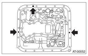
7) Install the oil pan by equally tightening the bolts.
