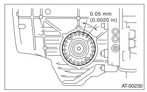
8) Turn the drive pinion several rotations with ST1 and check to see if the backlash is within the standard value with ST2, ST3, ST4 and ST5.
