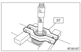
3) Remove the snap ring, and pull out the shaft from the center differential assembly.
