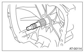
4) Remove the clip from torque converter clutch.
