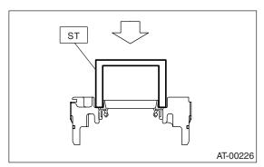
3) Apply gear oil to new O-ring and install it.
