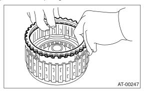
(2) Apply compressed air intermittently to check for operation.
