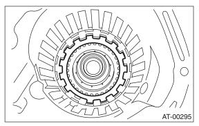
25) Turn the transmission case upside down, and then take out the socket bolts while holding the one-way clutch inner race with hand.
