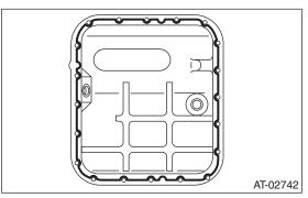
6) Apply liquid gasket fully to three holes other than screw holes on transmission case.
