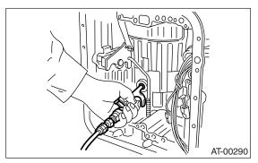
(4) Check the clearance between the retaining plate and the snap ring.
