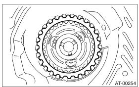
(2) Install a new 2-4 brake oil seal to transmission case.
