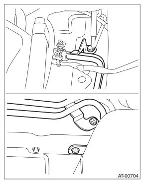
3) Connect ATF cooler hose to pipe transmission side.
