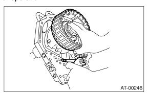
(4) Measure the clearance between the retaining plate and snap ring. (High clutch) At this time, do not press down retaining plate.
