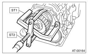
5) Pull out the shim(s) from transmission case.
