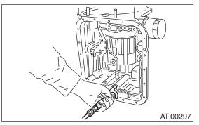
16) Place the same thickness of shim on both sides to prevent the plate from tilting, and then measure and record the clearance "B".
