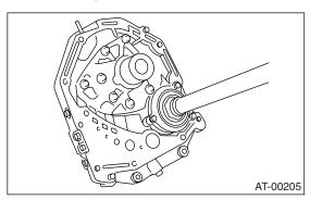
5) Rotate the drive pinion several times with ST1 and ST2.
