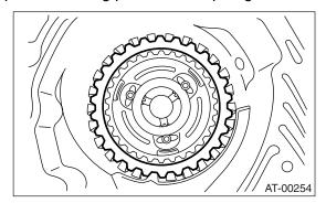
(8) Install a new 2-4 brake oil seal to transmission case.
