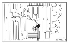
(9) After all 2-4 brake component parts have been installed, blow air intermittently and confirm the operation of brake.
