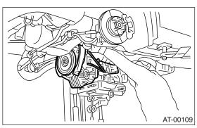
35) Separate the transmission assembly and rear cushion rubber.
