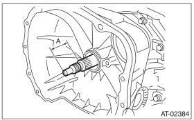
11) Install the torque converter clutch assembly. <Ref. to 4AT-81, INSTALLATION, Torque Converter Clutch Assembly.>
