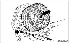
(9) Measure and record the clearance "B" between the retaining plate and snap ring. (Reverse clutch)
