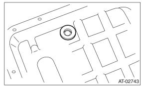
5) Apply proper amount of liquid gasket to the entire oil pan mating surface.
