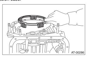
21) Position snap ring in transmission. Using ST, press the snap ring into place.
