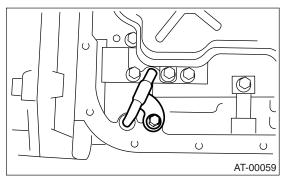
13) Remove the control valve body.
