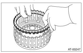
(8) Apply compressed air intermittently to check for operation.
