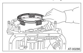
21) Remove the 2-4 brake piston and piston retainer without damaging.
