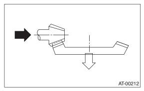
6) If tooth contact is correct, mark the retainer position and loosen it. After fitting a new O-ring and oil seal, screw in the retainer to the marked position. Then tighten the lock plate to the specified torque.
