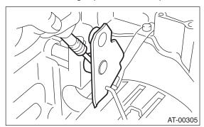
12) Remove bolt securing select lever, then remove select lever, manual plate and parking rod.
