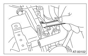
12) Install the ST to converter case. ST 498277200 STOPPER SET
