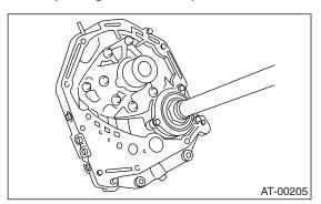
3) Rotate the drive pinion several times with ST1 and ST2.
