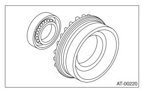
3) Take out either split pin, remove claw. ST 398527700 PULLER ASSY
