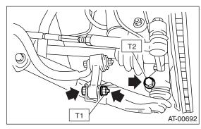
23) Install the shift select cable onto select lever. <Ref. to CS-26, INSTALLATION, Select Cable.>
