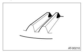
Corrective action: Decrease thickness of drive pinion height adjusting washer in order to move drive pinion away from hypoid driven gear.
