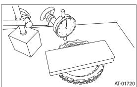
(5) Using the following formula, calculate N indicated on the push/pull gauge.
