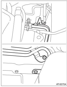
8) Remove the oil cooler inlet and outlet pipes.
