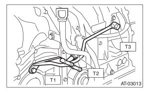
2) Install ATF cooler pipe to frame.
