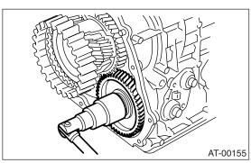
6) Using the ST1 and ST2, extract the reduction driven gear.
