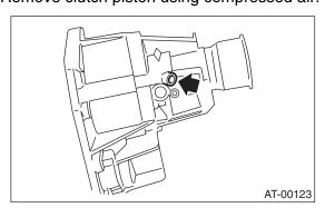
4) Pay attention, not to deform pipe, and remove transfer clutch pipe.
