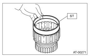
5) Set the cover on the piston with a press using ST1 and ST2, and attach the snap ring. At this time, be careful not to fold cover seal during installation.
