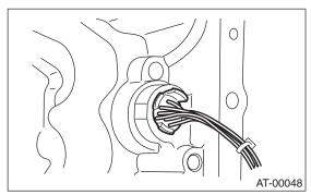
2) Connect the harness connectors. Connect the connectors of same color, and secure the connectors to valve body using clips. (Turbo model)
