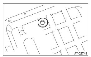
6) Apply proper amount of liquid gasket to the entire oil pan mating surface.
