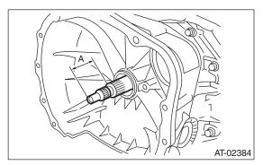
12) Install the torque converter clutch assembly. <Ref. to 4AT-81, INSTALLATION, Torque Converter Clutch Assembly.> 13) Install the transmission assembly to the vehicle. <Ref. to 4AT-44, INSTALLATION, Automatic Transmission Assembly.>
