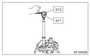
6) Tighten the LH retainer until contact is felt while rotating the shaft. Then loosen the RH retainer. Keep tightening the LH retainer and loosening the RH retainer until the pinion shaft can no longer be turned. This is the "zero" state.
