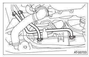
6) Disconnect ATF cooler hoses from pipes.
