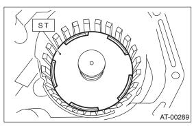
22) Install planetary gear and low clutch assembly to transmission case.
