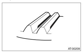
Corrective action: Reduce thickness of drive pinion height adjusting washer in order to move drive pinion away from hypoid driven gear.
