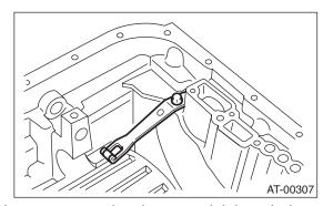
2) Insert range select lever, and tighten bolt.
