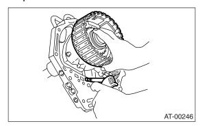
(10)Measure and record the clearance "B" between the retaining plate and snap ring. (High clutch)
