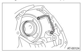
4) Apply ATF to new O-ring and install the test plug.
