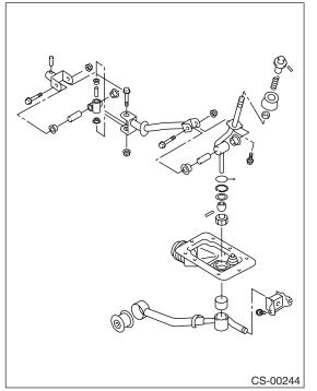
2) Check the swing torque of the rod in relation of the gear shift lever.
