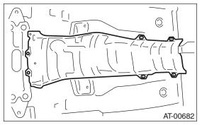
8) Install the front, center, rear exhaust pipe and muffler. (SOHC model)
