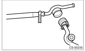
13) Remove the boot and bushing from gear shift lever.
