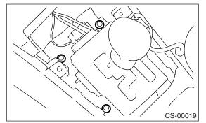
3) Install the console box. <Ref. to EI-47, INSTAL-LATION, Console Box.>
