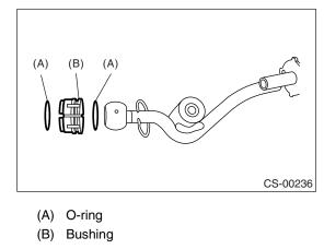
14) Remove the spring pin, and then remove the bushing and snap ring.
