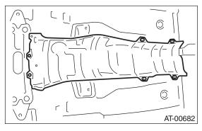
9) Remove the stay from transmission bracket.
