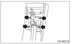
9) Install the console box. <Ref. to EI-47, INSTAL-LATION, Console Box.>
