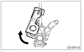
17) Remove the bushing from bracket.
