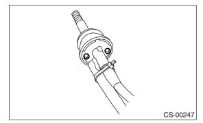
6) Fix the slider and reverse check cable end with spring pin.
