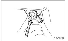
3) Move the transmission to right side, and then install the joint COMPL and stay.
