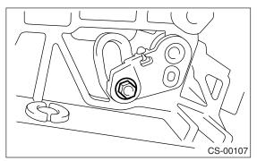
9) Remove the lock plate A, B, C and bushing.
