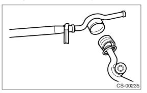
6) Install the washer and snap ring.
