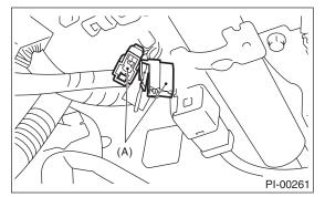
5) Connect the Subaru Select Monitor to data link connector.
