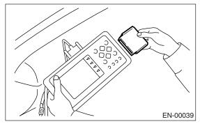
6) Connect the test mode connector (A) at the lower portion of instrument panel (on driver's side).
