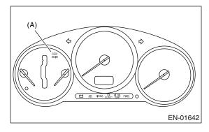
2) After starting the engine, the malfunction indicator light goes out. If it does not, either the engine or the emission control system is malfunctioning.
