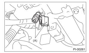
7) Connect the Subaru Select Monitor to data link connector.
