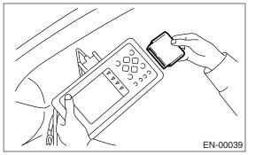
4) Connect the test mode connector (A) at the lower portion of instrument panel (on driver's side).
