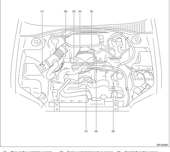
(1) Mass air flow and intake air temperature sensor
