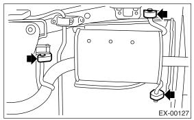
3) Remove the front, right and left cushion rubber, and detach the muffler assembly.
