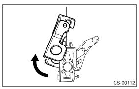
17) Remove the bushing from bracket.
