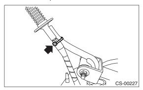
4) Remove the reverse check cable from cable plate.
