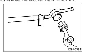
13) Remove the boot and bushing from gear shift lever.
