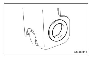
16) Remove the bracket from select lever assembly.
