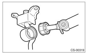
6) Remove the boot, bushing and snap ring from gear shift lever.
