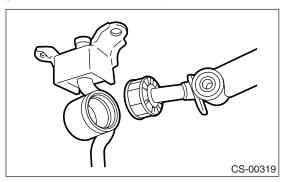
7) Install the washer and snap ring.
