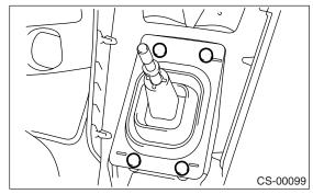
6) Remove the boot and insulator assembly.
