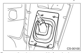
7) Remove the plate assembly from body.
