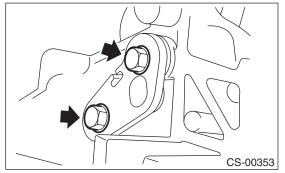
9) Remove the lock plates A, B, C and bushing.
