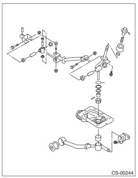
2) Check the swing torque of the rod in relation of the gear shift lever.
