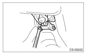
3) Move the transmission to right side, and then install the joint COMPL and stay.
