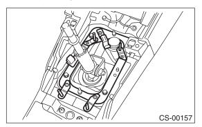
12) Pay attention to the direction of boot and insulator assembly and install them to the vehicle.
