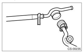
6) Install the washer and snap ring.
