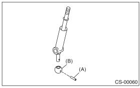
5) Apply grease to the bushing and O-ring, and then install to the gear shift lever.
