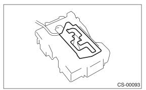
11) Remove the clip, and then remove the "P" range switch.
