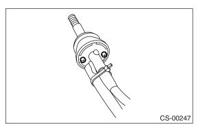
3) Fix the slider and reverse check cable end with spring pin.
