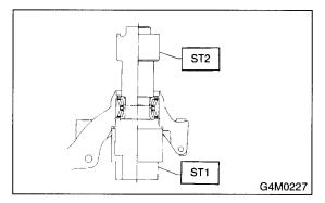
8) Using ST and a hydraulic press, drive hub bolts out.
