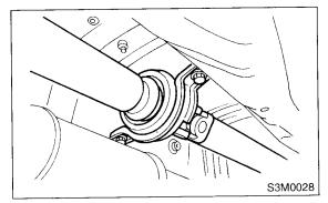
2) Align the matching marks and connect the flange yoke and rear differential.
