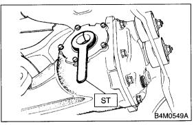
11) Insert the DOJ spline end into the bore of side oil seal, and remove ST.
