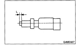
2) Measure the clearance between threaded end of stop light switch and stopper.
