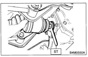
12) Align the DOJ and differential splines.
