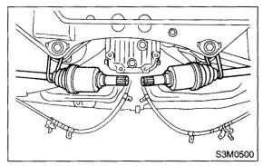
16) Remove the lower differential bracket.
