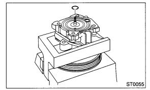
3) Extract the oil pump pulley from the front casing.
