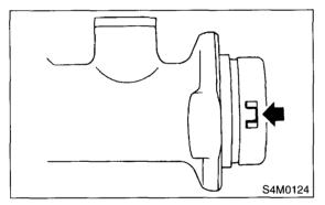
4) Install the seal to reservoir tank.
