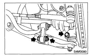
5) Tighten the following points in the order shown below when the wheels are in full contact with the ground and vehicle is curb weight.
