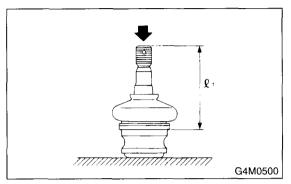
(2) With 686 N (70 kgf, 154 lb) loaded in the opposite direction shown in the figure, measure dimension  $\ell_2$ .
