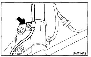
5) Remove the bolts which secure sensor harness to body.
