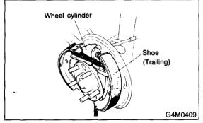
7) Fix the shoes by connecting hold-down cup to hold-down pin.
