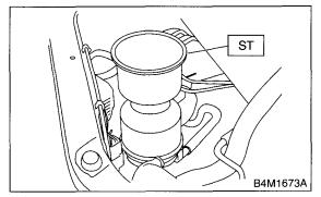
2) Continue to turn the steering wheel slowly from lock to lock until the bubbles stop appearing in the tank while keeping the fluid at that level.
