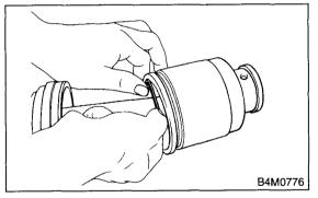
4) Remove the SFJ outer race from shaft assembly.
