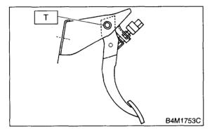
4) Set the brake pedal position by adjusting the position of stop light switch.
