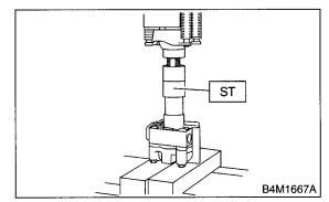
4) Install the pump pulley to front body.
