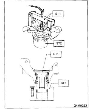
If inner bearing race remains in the hub, remove it with a suitable tool (commercially available).
