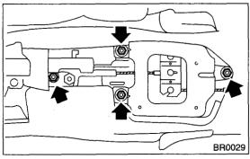
7) Roll up the floor mat and remove clamps.
