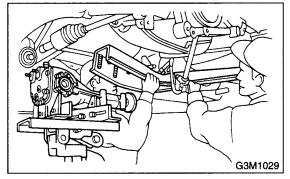
2) Insert the DOJ of rear drive shaft into rear differential.<Ref. to DI-37, REPLACEMENT, Rear Differential Side Oil Seal.>
