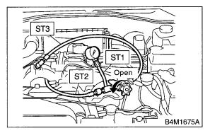
Service limit: TURBO model 7,350 — 8,036 kPa (75 — 82 kg/cm<sup>2</sup>, 1,067 — 1,165 psi) Non-TURBO model 7,164 — 7,840 kPa (73 — 80 kg/cm<sup>2</sup>, 1,040 — 1,137 psi) (4) If it is within the specified value, measure the steering effort. <Ref. to PS-78, MEASURE-MENT OF STEERING EFFORT, INSPECTION, General Diagnostic Table.> If it is not within specified value, replace the control valve itself or control valve and pinion as a single unit with new ones.
