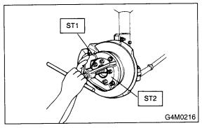
8) Remove the disc rotor from the hub. If disc rotor seizes up within hub, drive disc rotor out by installing an 8-mm bolt in screw hole on the rotor.
