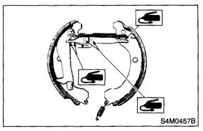
4) Connect the upper shoe return spring to shoes.5) Connect the parking brake cable to parking lever.
