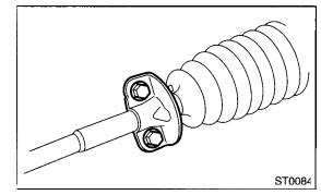
4) Remove the tie-rod end and lock nut from the gearbox.
