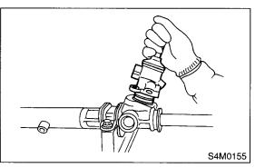
14) Using a sharp pointed pliers, rotate the rack stopper in the direction of the arrow until the end of the circlip comes out of the stopper. Rotate the circlip in the opposite direction and pull it out.
