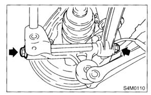
12) Disengage the BJ from the housing splines, and remove the rear drive shaft assembly. If it is hard to remove, use STs.
