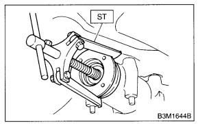
12) Remove the oil seal using ST. ST 499705401 PULLER ASSY
