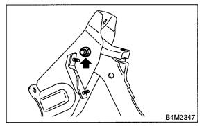
3) Remove the bush, spacer and spring.
