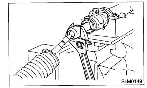
11) Loosen the adjusting screw and remove the spring and sleeve.
