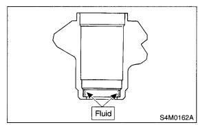
3) Attach ST2 to ST1, and press the oil seal into the place using a press.
