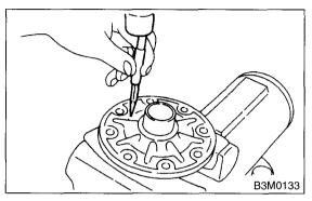
11) Draw out the pinion mate shaft and remove pinion mate gears, side gears and thrust washers. (Without LSD)
