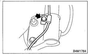
5) Remove the two bolts securing housing to strut.
