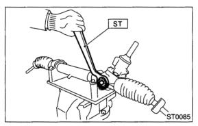
4) Tighten the adjusting screw until it no longer tightens.
