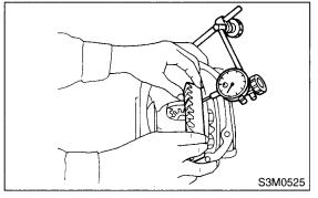
17) Checking and adjusting the tooth contact of crown gear:
