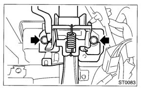
11) Pull out the steering shaft assembly from the hole on toe board.
