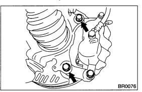
5) Remove the disc rotor.
