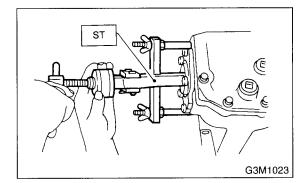
11) Drive in a new side oil seal with ST.
