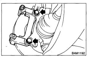
8) Clean mud and foreign particles from the caliper body assembly and support.
