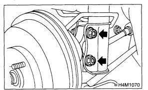
7) Remove the nuts securing strut mount to body.
