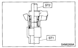
9) Apply the sufficient grease to oil seal lip.
