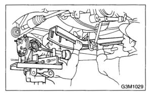
22) Remove the rear differential from front member, and remove rear member.
