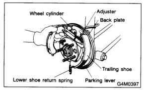
8) Disconnect the parking brake cable from parking lever.
