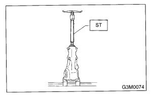
15) Remove the rear bearing cone from drive pinion by supporting cone with ST.
