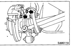
6) Raise the caliper body and move it toward the vehicle center to separate it from support.
