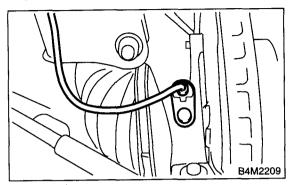
2) Install the front ABS sensor on strut and wheel apron bracket.
