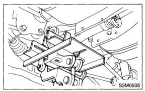
18) Remove the self-locking nuts and bolts.
