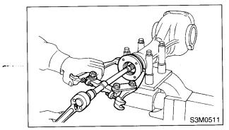
14) Press the end of drive pinion shaft and extract it together with rear bearing cone, preload adjusting spacer and washer.
