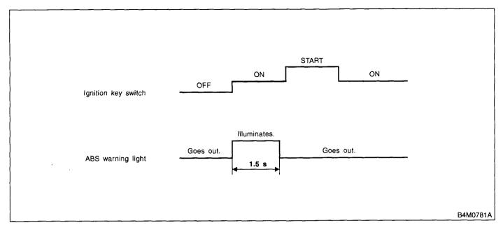
1) When the ABS warning light does not illuminate in accordance with this illumination pattern, there must be an electrical malfunction.
