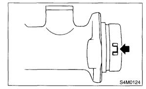
4) Extract the primary piston assembly and secondary piston assembly.
