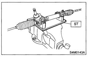
3) Using ST, loosen the lock nut. ST 926230000 SPANNER
