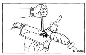
5) Loosen the adjusting screw and remove the spring and sleeve.
