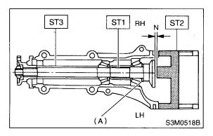
(A) Pinion height adjusting shim
