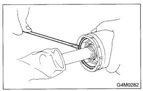
11) Apply an even coat of the specified grease [20 to 30 g (0.71 to 1.06 oz)] to the entire inner surface of boot. Also apply grease to shaft.
