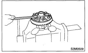
13) Press the side bearing cone onto differential case with ST.
