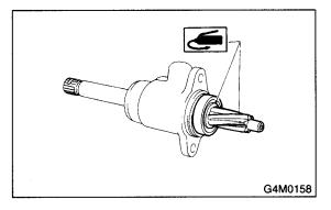
18) Install the gasket on the valve assembly. Insert the valve assembly into the place while facing rack teeth toward pinion.
