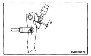
9) Apply grease to operating rod connecting pin to prevent it from wearing.
