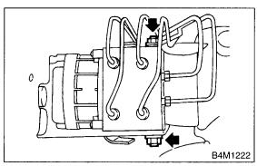
3) Connect the brake pipes to their correct AB-SCM&H/U connections.
