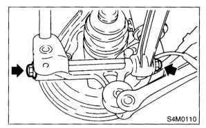
4) Connect the rear housing assembly to the trailing link assembly.
