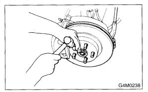
11) Install the wheel and tighten the wheel nuts to specified torque.
