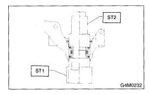
5) Using pliers, install the snap ring in its groove.
