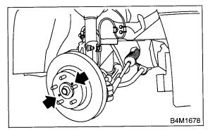
9) Remove the cotter pin and castle nut which secure tie-rod end to housing knuckle arm.
