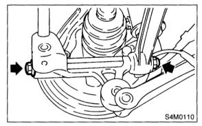
13) Disengage the BJ from the housing splines, and remove the rear drive shaft assembly.
