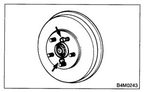
4) Hold the hold-down pin by securing rear of back plate with your hand.
