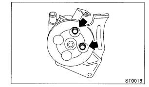
2) Tighten the bolt which install power steering pump bracket.
