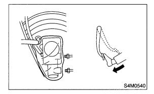
4) Close the outlet plug with your finger, and release the brake pedal.
