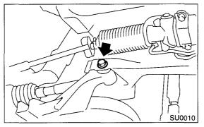
8) Remove the nuts attaching engine mount cushion rubber to crossmember.
