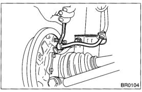
9) Disconnect the parking brake cable end.
