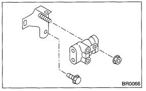
1) Remove the brake pipe from proportioning valve at four places.
