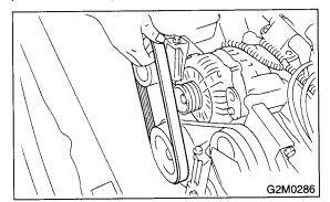
5) Disconnect the connector from the power steering pump switch. 6) Disconnect the pipe C and suction hose from the oil pump.
