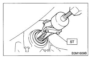
13) Fit a new oil seal using ST. ST 498447120 DRIFT
