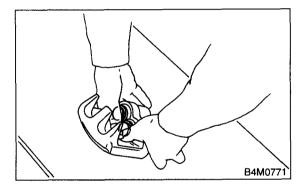
5) Apply a coat of specified grease to the boot and fit in the groove on ends of cylinder and piston.
