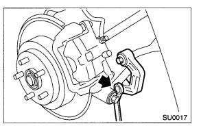
3) Remove the bolt which secures stabilizer to stabilizer bracket.
