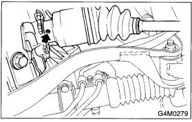
8) Remove the front drive shaft assembly. If it is hard to remove, use ST1 and ST2.
