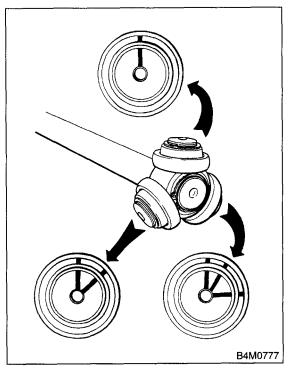
15) Align alignment marks on shaft and outer race, and install outer race.
