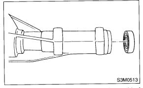
17) Remove the pilot bearing together with front bearing cone using ST.
