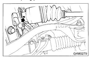
6) Remove the EBJ and SFJ boots from the drive shaft. <Ref. to DS-33, DISASSEMBLY, Front Drive Shaft.>
