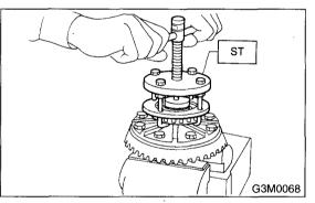
9) Remove the crown gear by loosening crown gear bolts.
