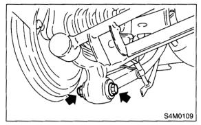
12) Remove the bolts which secure lateral link assembly to the rear housing.
