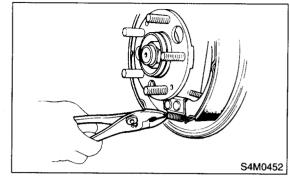
7) Remove the shoes one by one from back plate with adjuster.
