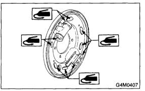
3) Apply grease to the adjusting screw and both ends of adjuster.
