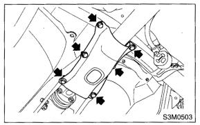
11) Remove the propeller shaft. <Ref. to DS-14, REMOVAL, Propeller Shaft.>
