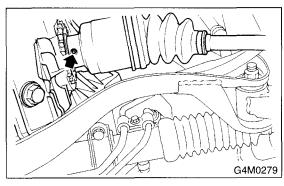
9) Connect the transverse link to the housing.10) Install the stabilizer link.
