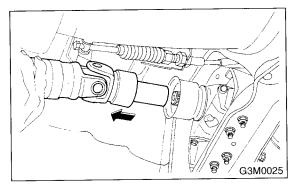
12) Install the extension cap to transmission.
