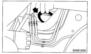
2) Insert the end of steering shaft into the toe board grommet.
