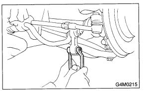
6) Remove the disc brake caliper from the housing, and suspend it from strut using a wire.
