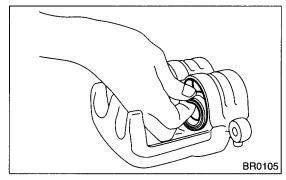
4) Remove the piston seal from caliper body sylinder.
