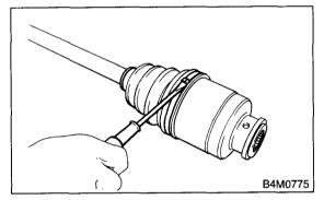
3) Remove the circlip from SFJ outer race using screwdriver.
