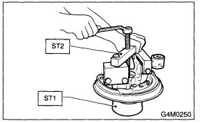
2) Remove the back plate from the rear housing3) Using a standard screwdriver, remove the outer and inner oil seals.
