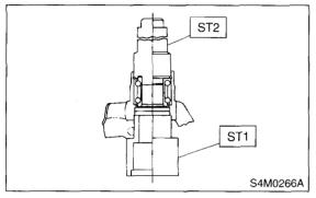
4) Using plier, install the snap ring.
