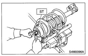
3) Remove the strut mount, upper spring seat and rubber seat from strut.
