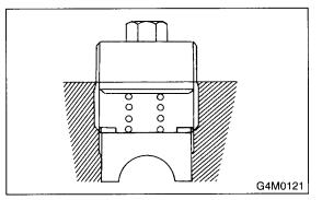
(5) Apply liquid packing to at least 1/3 of entire perimeter of adjusting screw thread.
