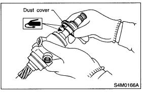
16) Install the dust cover on the valve assembly.17) Apply genuine grease to the pinion gear and bearing of valve assembly.
