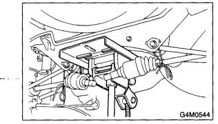
5) Remove the bolts securing crossmember to vehicle body, and remove the crossmember.
