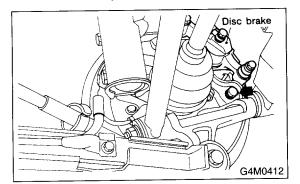
3) Suspend the disc brake assembly so that the hose is not stretched.
