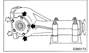
(6) Measure the crown gear-to-drive pinion backlash. Set the magnet base on differential carrier. Align the contact point of dial gauge with tooth face of crown gear, and move crown gear while holding drive pinion still. Read the value indicated on dial gauge.
