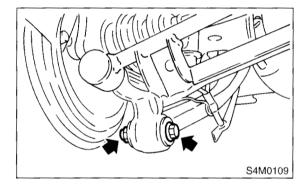
11) Remove the bolts which secure lateral assembly to the rear housing.
