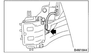
3) Secure the middle fitting of brake hose to bracket at strut location using a clamp.
