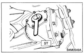
5) Insert the DOJ spline end into the bore of side oil seal, and remove ST.
