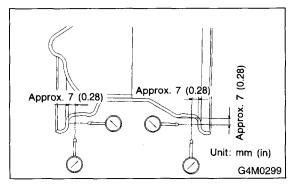
4) If the rim runout exceeds specifications, remove the tire from rim and check runout while attaching dial gauge to positions shown in figure.5) If the measured runout still exceeds specifica-
