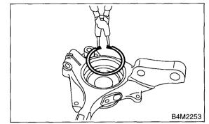
6) Using ST1 and ST2, press the outer oil seal until it contacts the bottom of housing.
