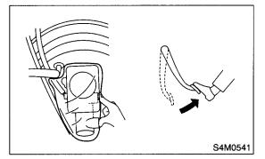
5) Repeat the above step3) and 4) until brake fluid is completey bled from outlet plug.
