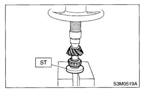
5) Insert the drive pinion into differential carrier, install the previously selected bearing preload adjusting spacer and washer.
