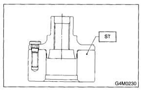
2) Remove the foreign particles (dust, rust, etc.) from the mating surfaces of hub tone wheel, and install the tone wheel to hub (only vehicle equipped with ABS).
