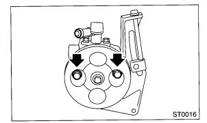
9) Remove the bolt from the rear side of oil pump.
