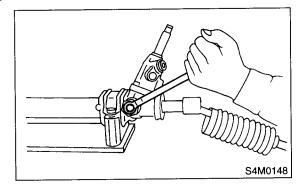
10) Using a wrench [32 mm (1.26 in) width across flats] or adjustable wrench, remove the tie-rod.
