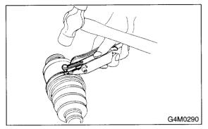
17) Cut off the band with an allowance of about 10 mm (0.39 in) left from the clip and bend this allowance over the clip.
