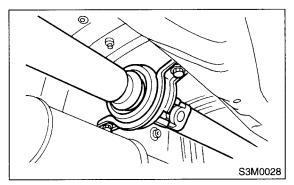
11) Remove the propeller shaft from the transmission.
