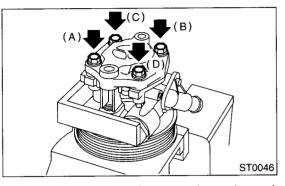
11) When the reassembly procedures have been completed, turn the shaft by hand to ensure it turns smoothly. If it binds or other unusual conditions are evident, disassemble again and check for foreign matter trapped on sliding surfaces and improper installation. Eliminate the cause of trouble.
