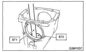
(2) Insert the ST1 into carrier with pinion height adjusting washer and rear bearing cone fitted onto it.
