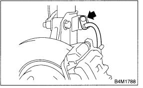
3) Scribe an alignment mark on the camber adjusting bolt which secures strut to housing.4) Remove the bolt securing the ABS sensor harness.
