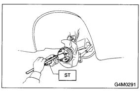
3) Tighten the axle nut temporarily.
