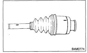
16) Install the circlip in the groove on the SFJ outer race.
