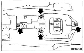
7) Remove the inner cable end from equalizer.
