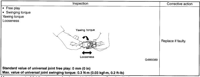
Measurement of folding torque of universal joint is as shown in the figures.
