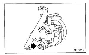
2) Tighten the bolt which installs power steering pump bracket.
