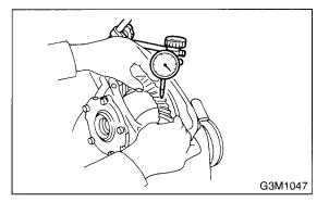
(7) At the same time, measure the turning resistance of drive pinion. Compared with the resistance when differential case is not installed, if the increase of the resistance is not within the specified range, readjust side bearing retainer shims.
