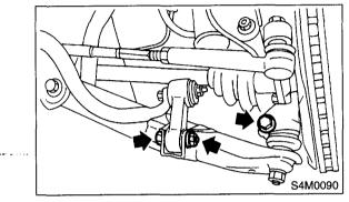
7) Remove the nut (do not remove bolt.) securing the transverse link to crossmember.
