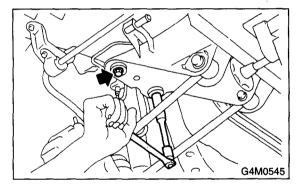
6) Scribe an alignment mark on the rear lateral link cam bolt and crossmember.
