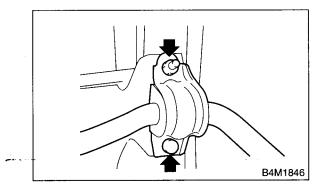
5) Remove the bolts which secure the stabilizer link to front transverse link.
