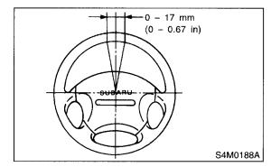
4) If the steering wheel spokes are not horizontal with vehicle set in the straight ahead position after this adjustment, correct it by turning the right and left tie-rods in the same direction by the same turns.
