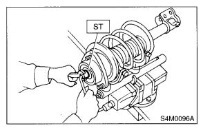
10) Loosen the coil spring carefully.
