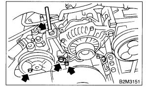
7) Place the oil pump bracket in a vise, remove the two bolts from the front side of oil pump.
