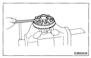
10) Drive out the pinion shaft lock pin from crown gear side. (Without LSD)
