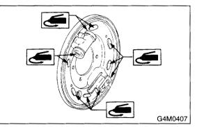
4) Install the brale assembly on hopusing, and tighten bolts to install the back plate.
