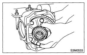
7) When replacing the side bearing, pull the bearing cup from side bearing retainer using ST. ST 398527700 PULLER ASSY
