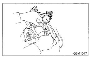
16) Check the crown gear runout on its back surface, and make sure pinion and crown gear rotates smoothly.
