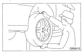
2) Inspect the lean of axis direction using a dial gauge. Replace the hub bearing if the load range exceed the limitation.
