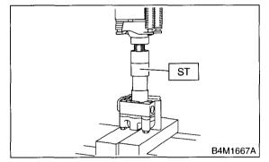
4) Press-fit the shaft assembly into the front body.5) Apply the specified hydraulic oil to the O-rings and fit them into the front casing.
