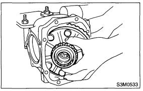
(3) Install the side retainer shims and O-rings to the left and right retainers from which they were removed.
