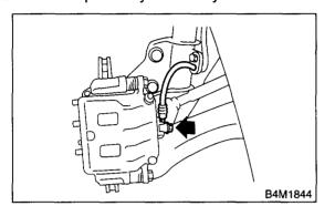
5) Remove the bolt securing lock pin to caliper body.
