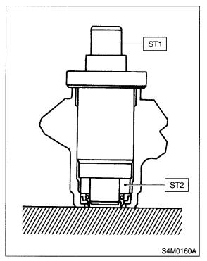
4) Using ST and press, install the special bearing in valve housing.
