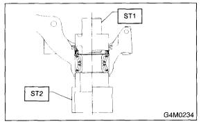
8) Invert the ST and housing. ST 927400000 HOUSING STAND 9) Apply the sufficient grease to oil seal lip.
