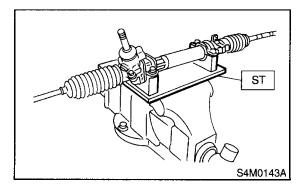
3) Remove the tie-rod end plate.
