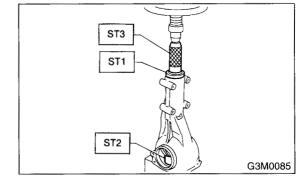
7) Insert the spacer, then press-fit pilot bearing with ST1 and ST2.
