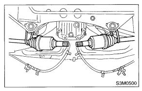
10) Remove the nut of protector. ST 398527700 PULLER ASSY
