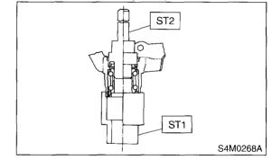
8) Using ST1 and ST2, press the sub seal into place.
