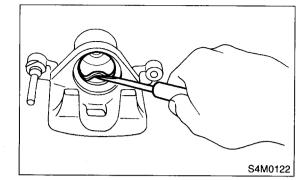
5) Remove the lock pin sleeve and boot from caliper body.
