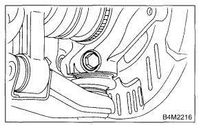
13) After scribing an alignment mark on camber adjusting bolt head, remove bolts which connect housing and strut, and disconnect the housing from the strut.
