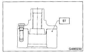
2) Using a hydraulic press, press the new hub bolts into place.
