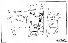
4) Install the rear differential protector. (If equipped)5) Install the rear exhaust pipe and muffler.
