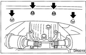
19) Remove the bolts which secure rear differential front member to body.
