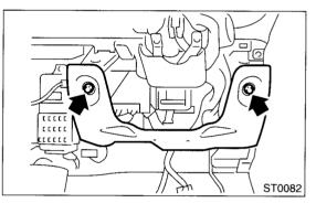
5) Connect all connectors under instrument panel. 6) Connect the airbag system connector at the harness spool.
