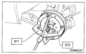
13) Remove the rear ABS sensor from the back plate (only vehicle equipped with ABS).
