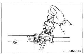
19) Tighten the bolts alternately to secure the valve assembly.
