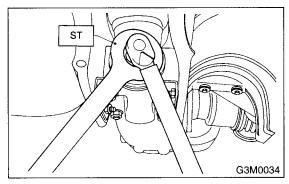
11) Extract the companion flange using ST. ST 399703602 PULLEY ASSY
