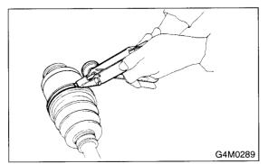
16) Tap on the clip with the punch provided at the end of ST.
