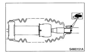
26) Using a screwdriver, tighten the screw until the ends "A" and "B" of the band come into contact with each other.
