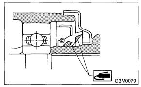
2) Adjusting preload for front and rear bearings: Adjust the bearing preload with spacer and washer between front and rear bearings. Pinion height adjusting washer are not affected by this adjustment. The adjustment must be carried out without oil seal inserted.
