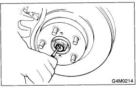
4) Remove the axle nut using a socket wrench.
