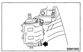
6) Raise the caliper body and move it toward the vehicle center to separate it from support.7) Remove the support from housing.
