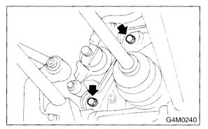
9) Install the rear ABS sensor and brake cable bracket (only vehicle equipped with ABS).
