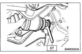
6) Align the DOJ and differential splines.
