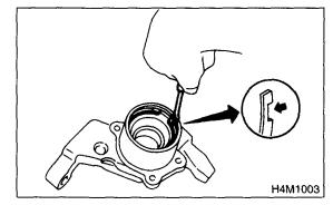
5) Using ST1 and ST2, remove the bearing by pressing inner race.
