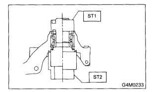
7) Using ST1 and ST2, press the inner oil seal until it contacts circlip.
