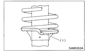
6) Install the helper and dust cover to the piston rod.
