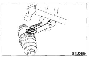
23) Cut off band with an allowance of about 10 mm (0.39 in) left from the clip and bend this allowance over the clip.
