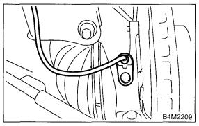
12) Remove the transverse link ball joint from the housing.
