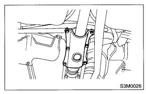
9) Remove the four bolts which hold propeller shaft to rear differential.
