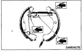
9) Install the brake shoe. <Ref. to BR-31, INSTAL-LATION, Rear Drum Brake Shoe.>
