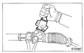
16) Tighten the bolts alternately to secure the valve assembly.
