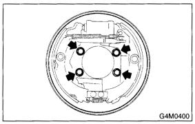
9) Remove the bolts installing the wheel cylinder on back plate, and remove it.
