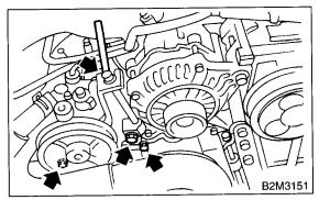
8) Place the oil pump bracket in a vise, remove the two bolts from the front side of oil pump.
