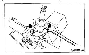
13) Carefully draw out the input shaft and remove the valve assembly.
