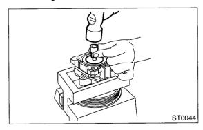
9) Install the O-ring to the rear cover.10) Install the rear cover.
