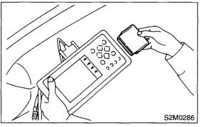
4) Connect the Subaru Select Monitor to data link connector.
