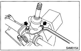
7) Carefully draw out the input shaft and remove the valve assembly.
