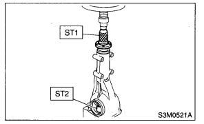
10) Install the self-locking nut. Then tighten it with ST.
