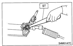
9) Tighten the adjusting screw until it no longer tightens.
