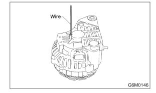
2) Heat the rear bracket [50 to  $60^{\circ}$ C (122 to 140°F)] and press the rear bearing into the rear bracket. Then lubricate the rear bracket.
