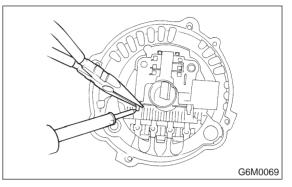
5) Remove the brushes by unsoldering at the pigtails.
