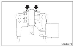
6) Remove the nut and insulating bushing at terminal B. Remove rectifier.
