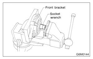
(3) Set a new bearing and closely install a fit tool on the bearing outer race. Press the bearing down into place with a hand press or vise. A socket wrench can serve as the tool.(4) Install front bearing retainer.
