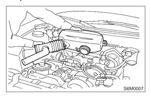
3) Remove air intake chamber stay. (AT vehicles only)
