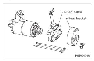
4) Remove armature and yoke. Ball used as a bearing will then be removed from the end of armature.
