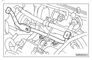
4) Disconnect connector and terminal from starter.
