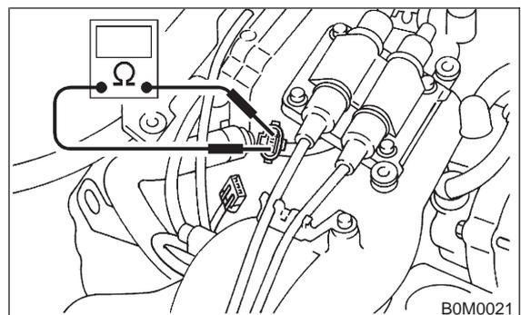
1) Check for open circuit. (range:  $\Omega \times 1K$ )
