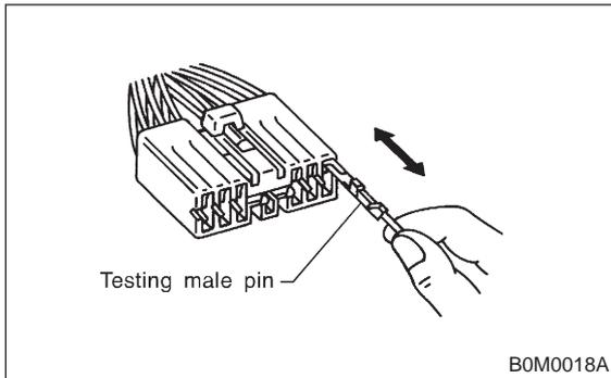
5) Shake lightly the connector and the harness, and check for sudden changes in voltage or resistance.
