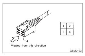
• The number of poles or pins, presence of a lock, and pin number of each terminal are indicated in the sketch of each connector. In the sketch, the highest pole number refers to the number of poles which the connector has. For example, the sketch of the connector shown in figure indicates the connector has 9 poles.
