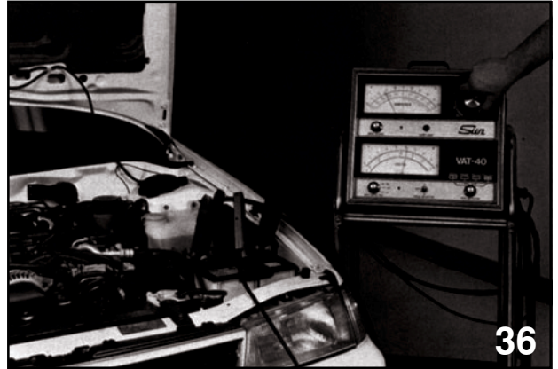
Battery performance test
