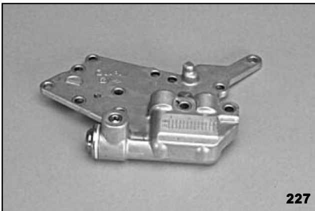
Relief Valve Case (Front Side)
