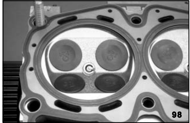
New Head Gasket Design
