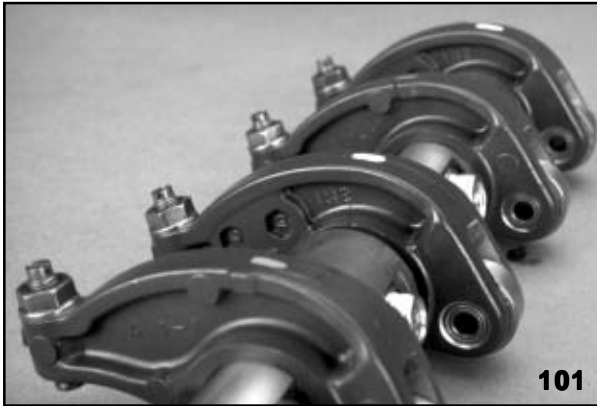
Adjustment Screw and Nut
