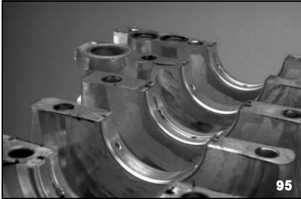
Main Bearing Oil Grooves
