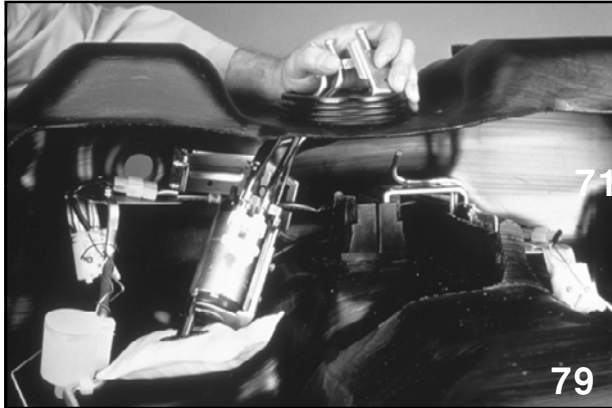
Removing Fuel Pump
