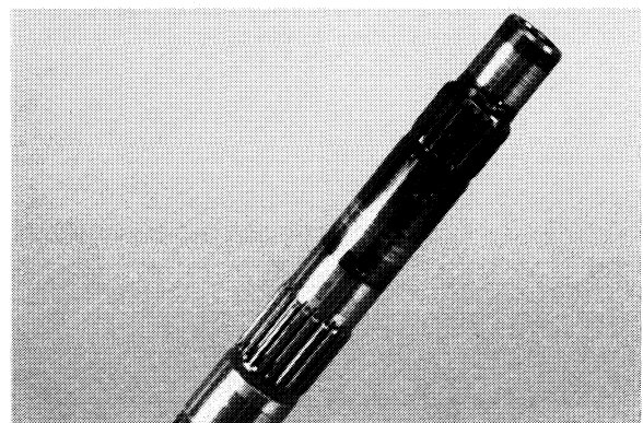
Discolored Input Shaft
