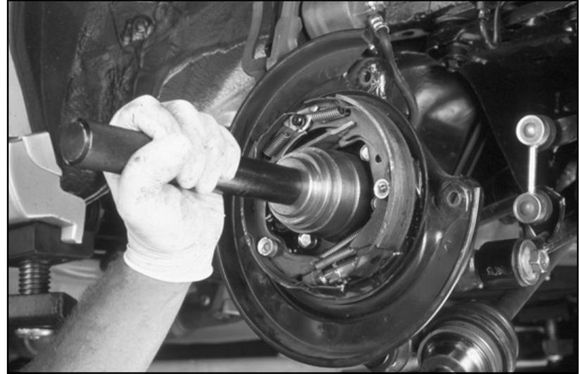
36. Remove all tools from the puller bolt. Push out the bearing stay from the center of the installed bearing using the head of the bolt.
