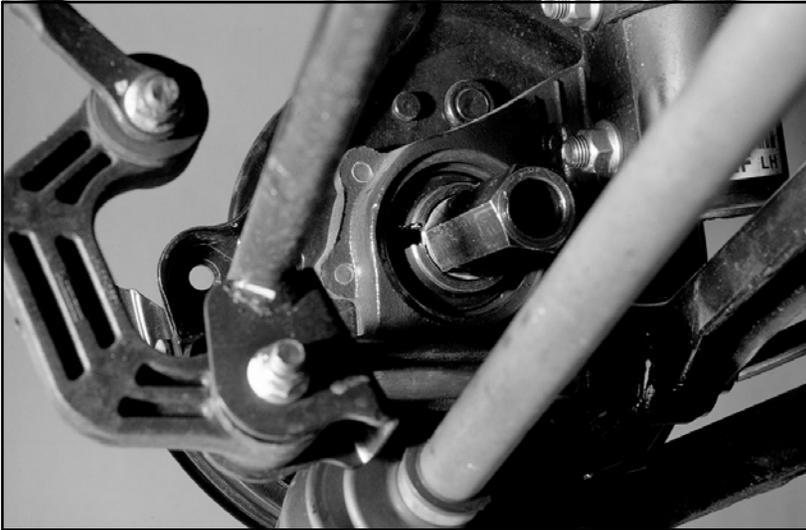
30. Secure the nut on the inner side with a wrench and begin tightening the bolt with an air ratchet.
