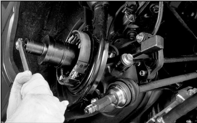
21. Switch to the air ratchet after the initial tension of the bearing has been overcome.
