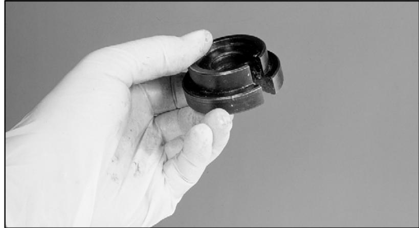
28. Front side of bearing housing with tools positioned for installation.
