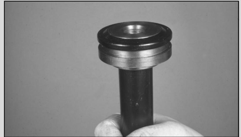
46. Reverse the J 45697-10 on the driver handle J 8092. Place the inner number two seal on the tool and install the seal. **The seal is fully installed when the seal is flush with the bearing housing.**
