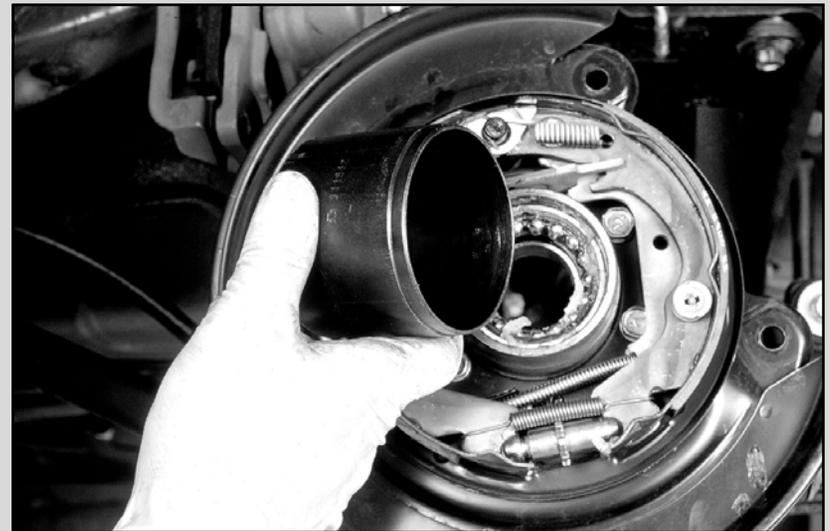
17. Place the OTC 314308 with a washer onto the puller bolt. This will be placed into the bearing housing. Apply the included special grease to the puller bolt, once during disassembly and again during reassembly.
