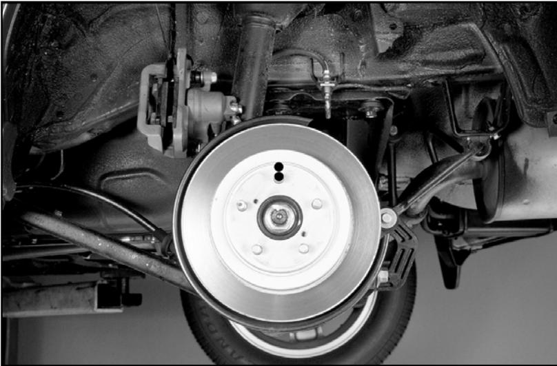
52. Stake Axle Nut. Then install the brake caliper mount and torque the bolts. Legacy, Impreza and Forester 38 ± 4 ft-lb
