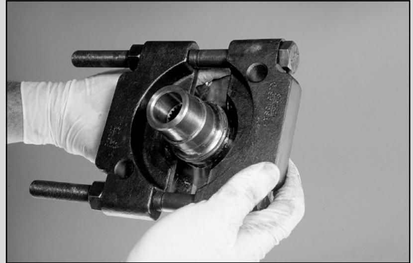
39. Install a set of press plates below the old inner race and remove with appropriate press and press tools.
