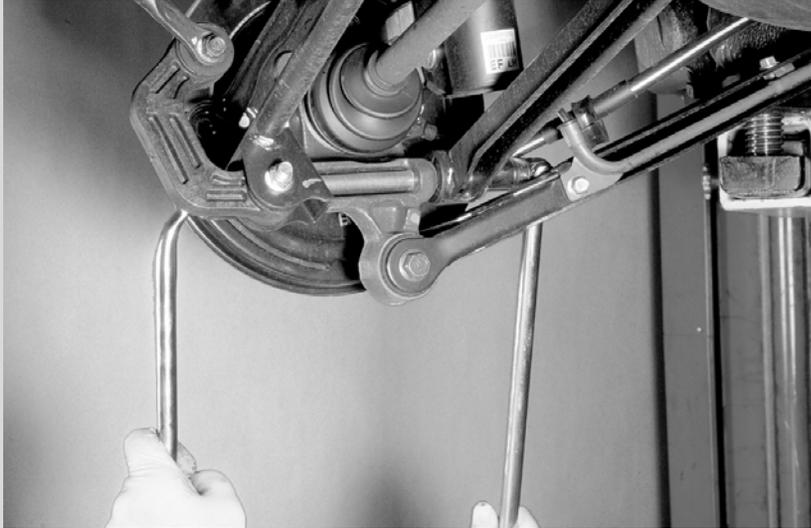
7. Push the bearing housing outward and slide the axle out.
