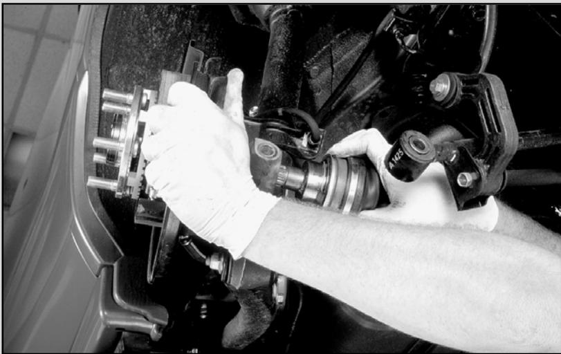
50. Install and torque the lateral link bolt. Use new self locking nut. **DO NOT USE IMPACT GUN.**
