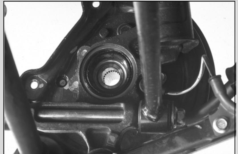
47. Check the rolling resistance of the hub with the supplied torque wrench. The hub should turn smoothly. (Starting force should be 7 to 17 inch pounds.)
