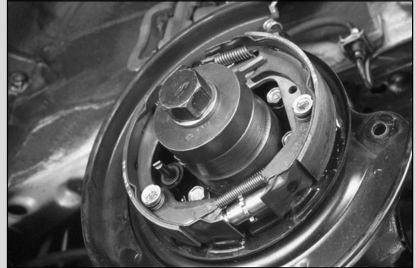
31. Tighten the last few turns with the breaker bar if necessary. Installation is complete when OTC 311888 makes contact with the bearing housing.
