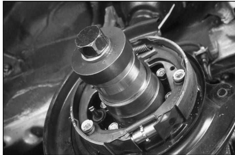
29. Back side of bearing housing positioned for bearing installation.
