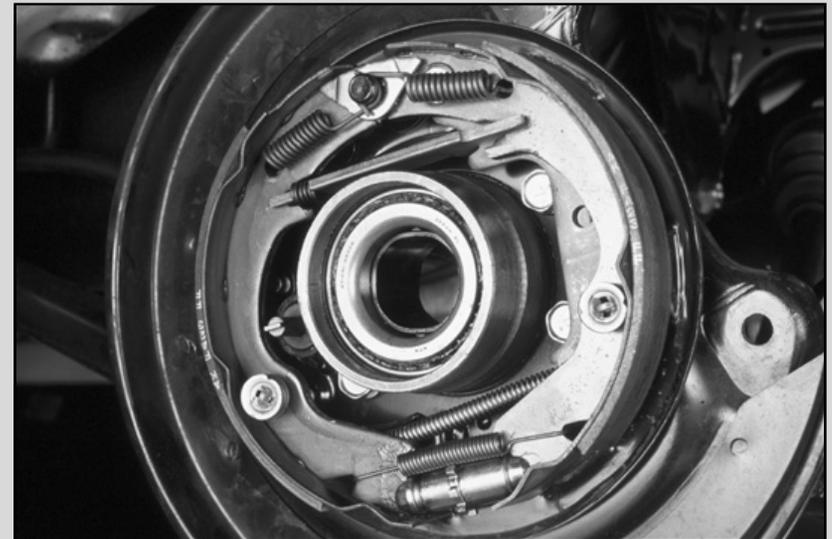
33. Insert the snap ring. If the snap ring will not seat properly the bearing is not fully installed.
