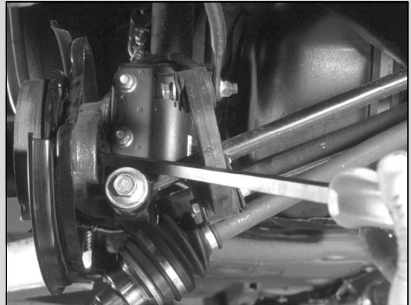
13. Place OTC 311882 over the bearing housing. The groove must face outward.
