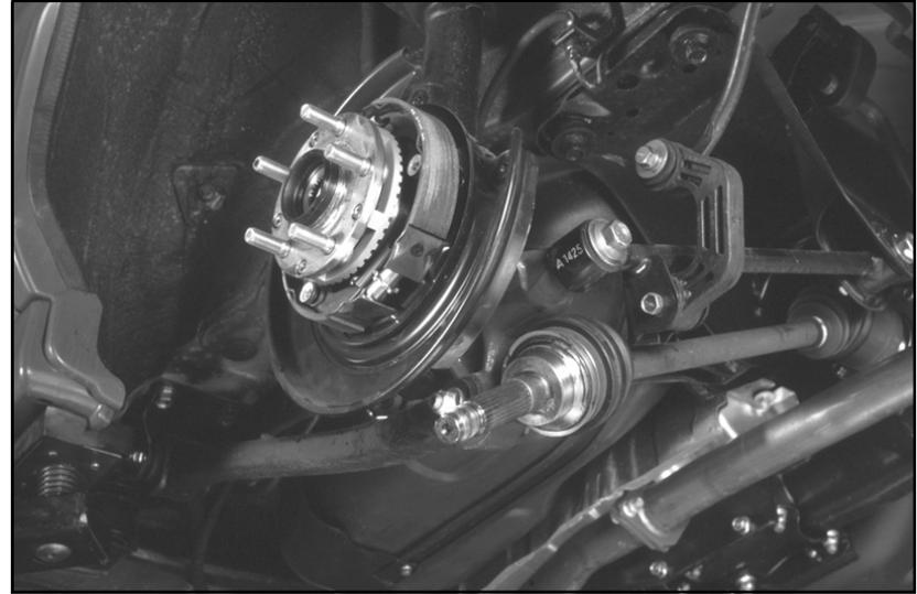
**(Inspect the axle for any deep scratches, pitting and damage to the dust shield. Replace if necessary.)**
