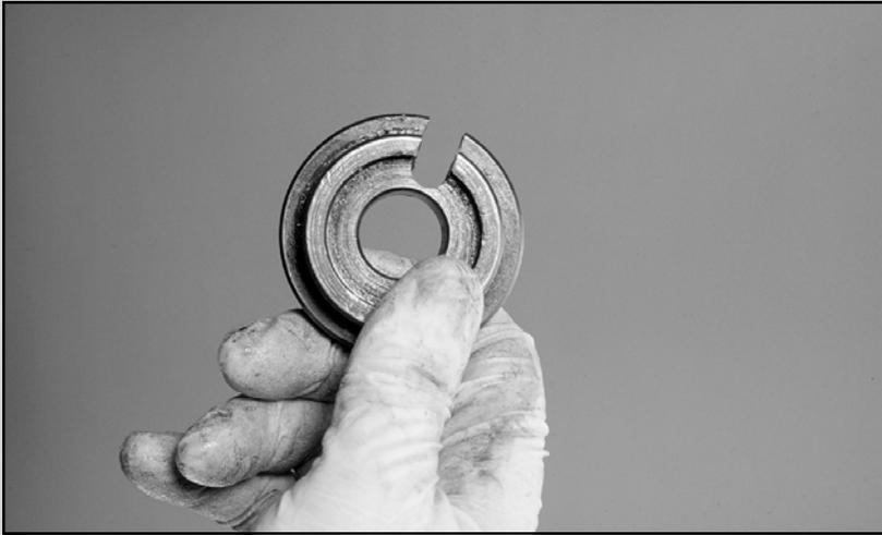
42. The slot will be used to insert a depth gauge.
