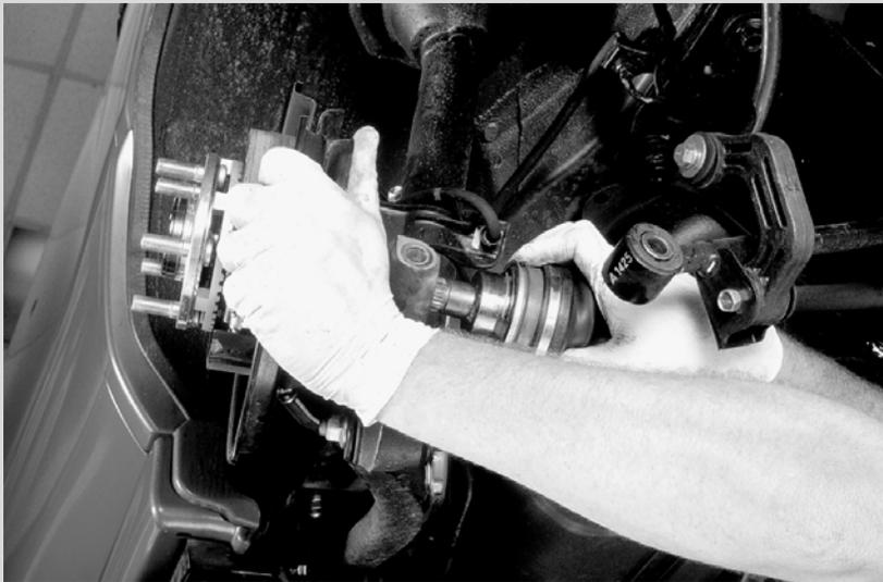
8. Set the axle below the lateral link bolt and reinstall the lateral link bolt.
