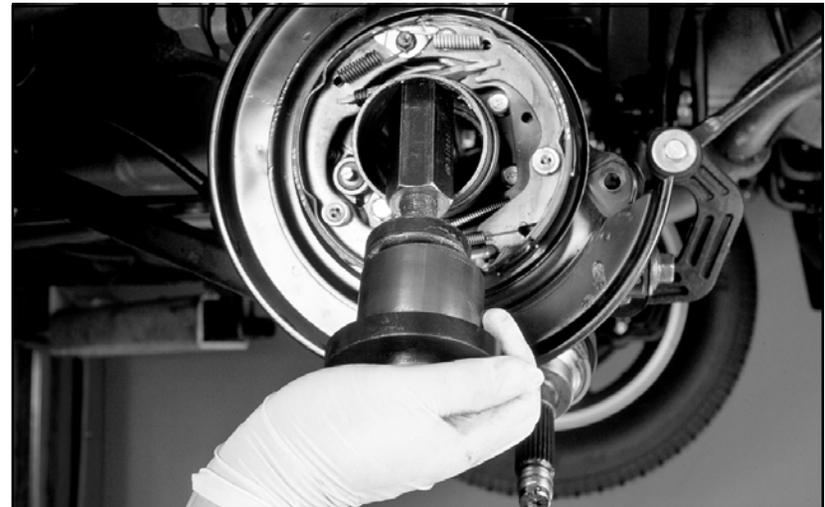
23. Clean and inspect the bearing housing for damage. Use the test outlined below to check for out of roundness condition. Replace bearing housing if out of round.
